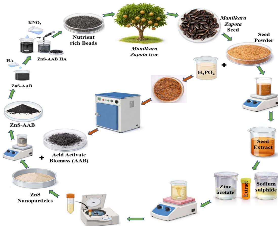
Fig. 1 Schematic of the synthesis of ZnS nanoparticles using Manilkara zapota seed extract, preparation of ZnS-loaded acid-activated biomass (ZnS-AAB), adsorption of humic acid, and subsequent conversion into nutrient-loaded alginate beads for controlled release applications.
