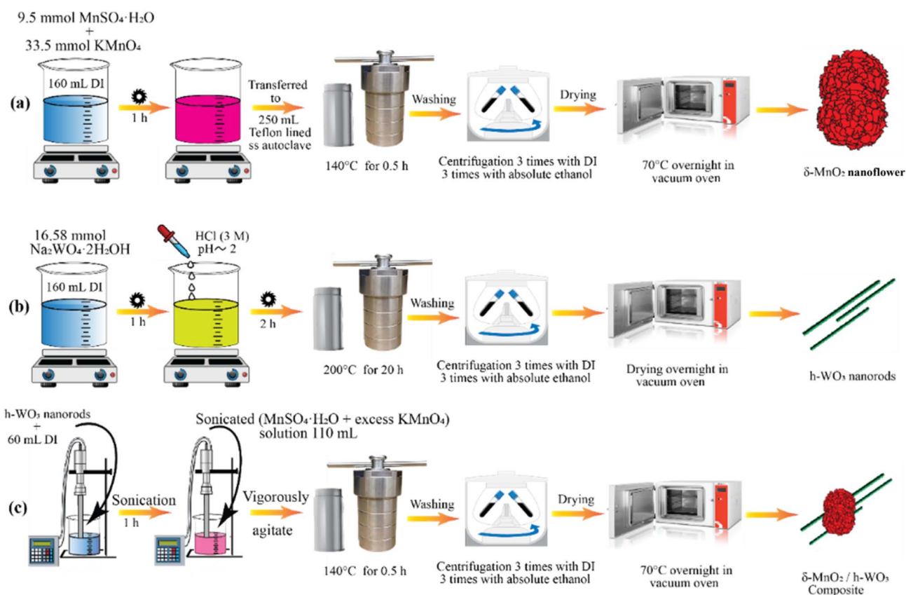
Fig. 1 Schematic diagram showing the step-by-step synthesis routes for \delta -MnO 2 (a), WO 3 (b), and \delta -MnO 2 /WO 3 (c) composite photocatalysts used in this study.
