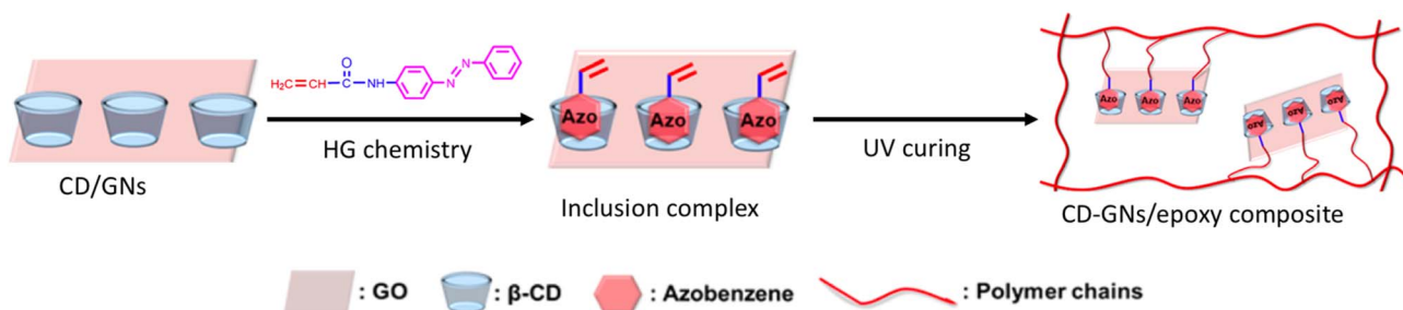
Fig. 6 Schematic of the preparation of self-healing CD-GN/epoxy composites; reproduced from ref. 81 with permission from the American Chemical Society, 81 copyright 2026.
