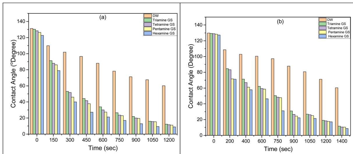
Fig. 18 The contact angle measurements with time for (a) sandstone and (b) carbonate rock samples.
