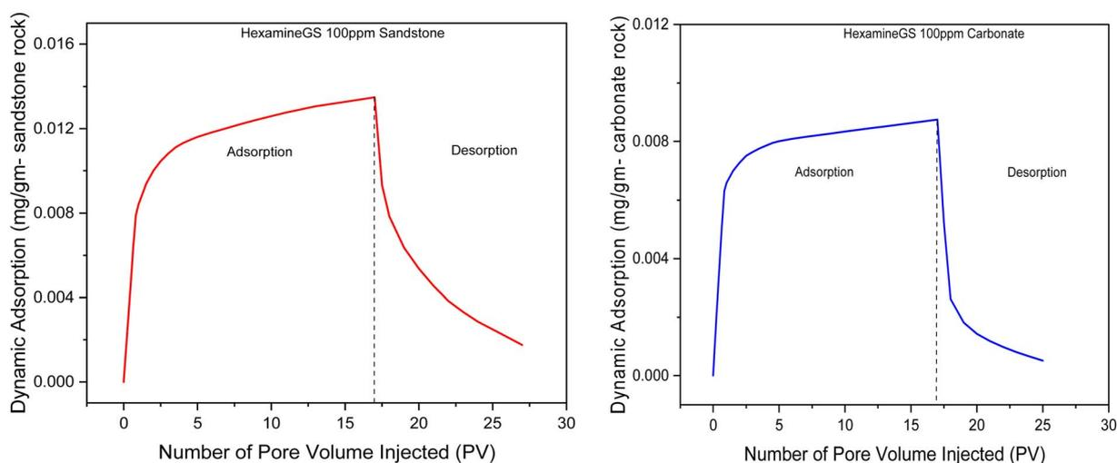
Fig. 17 Dynamic adsorption profile of Hexamine GS of sandstone and carbonate rock samples.
