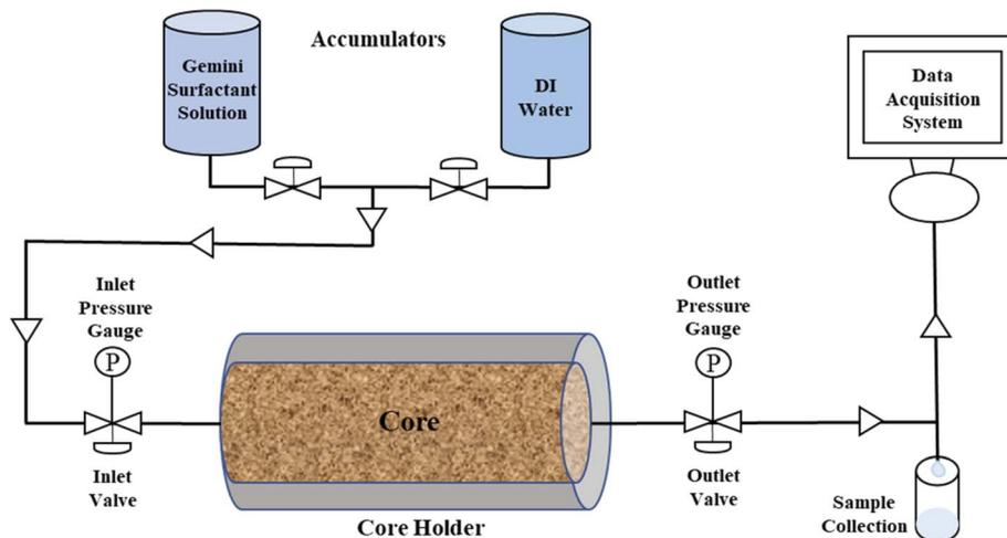
Fig. 3 Schematic of dynamic adsorption flooding system.
