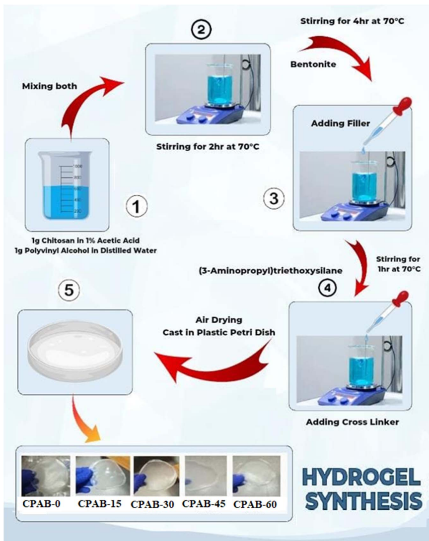
Fig. 1 Scheme for hydrogel synthesis and pictures of prepared CPAB hydrogels.
