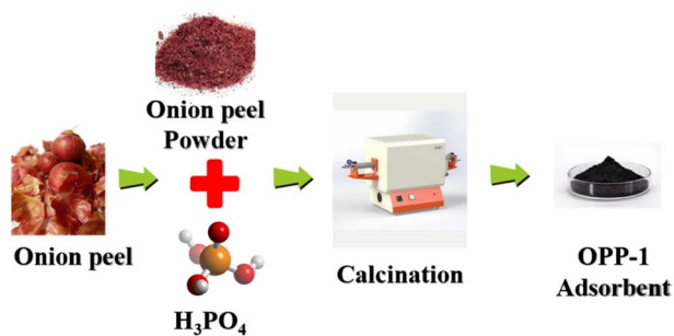
Fig. 1 Preparation of activated carbon derived from OP using orthophosphoric acid activation.
