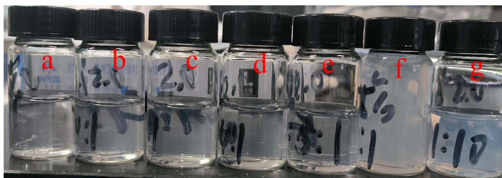
Fig. 11 Blended solutions of HX-36L and PDDN at different concentration ratios. Sample (a) is the blank containing 0.5% PDDN; samples (b) through (g) correspond to HX-36L : PDDN ratios from 10 to 0.1.
