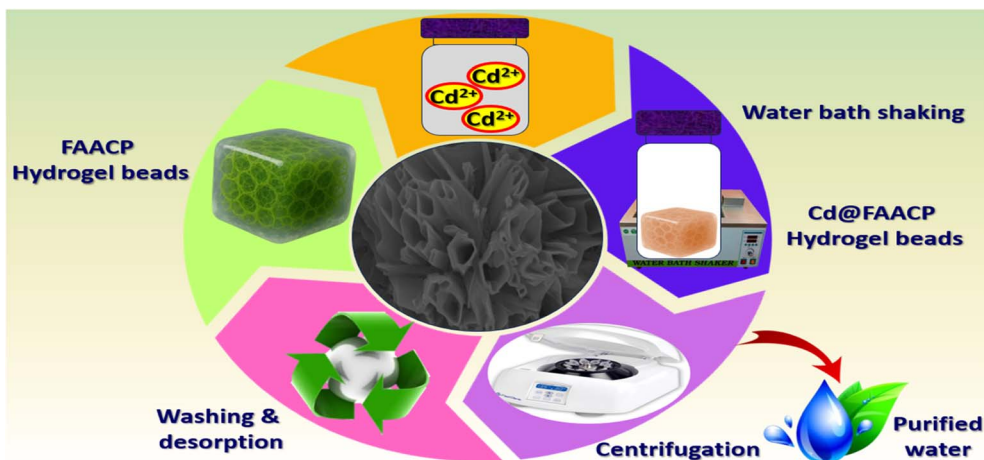
Fig. 1 A schematic diagram representing the capture and mechanism of Cd(II) ions removal by FAACP hydrogel beads.
