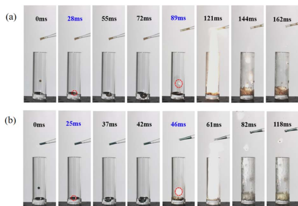
Fig. 7 Ignition delay times of (a) 10 wt% \text{Fe}(\text{vim})_2(\text{DCA})_2 + \text{IL} and (b) 10 wt% \text{Cu}(\text{vim})_2(\text{DCA})_2 + \text{IL} with \text{H}_2\text{O}_2 recorded using a high-speed camera (1000 fps).
