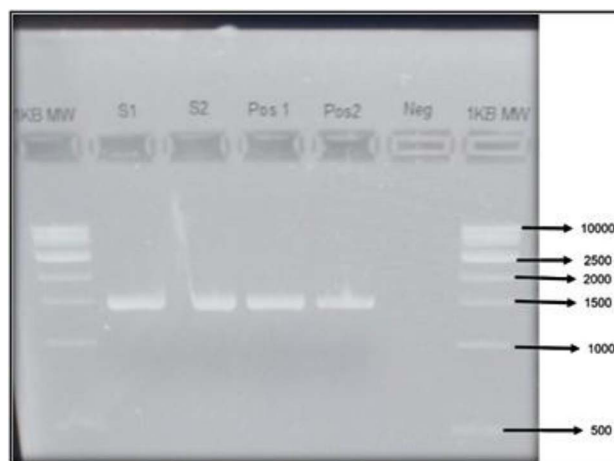
Fig. 10 Gel electrophoresis results. 1 KB MW is the 1 kb DNA ladder, 1% agarose, 1xTEA used, S1 and S2 are the DNA amplicons samples in duplicates, Pos2 and Neg are the positive and negative controls ( S. aureus ). The numbers on the right represent the base pairs.
