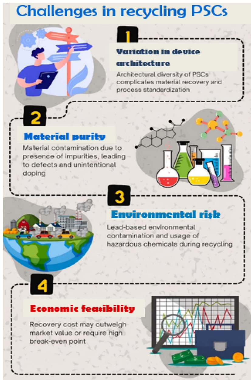
Fig. 9 Challenges in recycling of perovskite solar modules. 79
