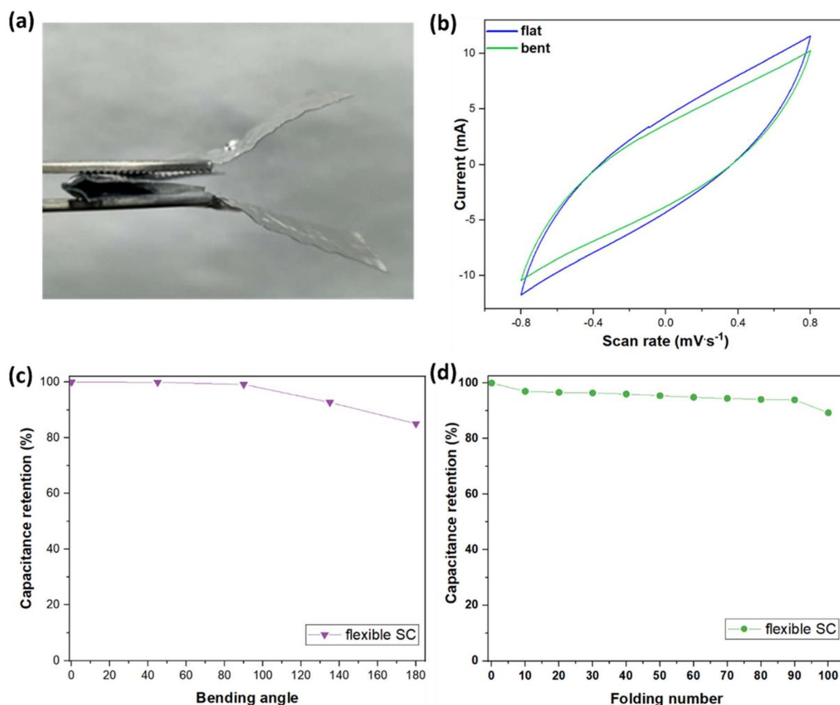
Fig. 9 (a) Photograph of the flexible supercapacitor, (b) cyclic voltammetry of the flexible SC measured at  $100\ mV\ s^{-1}$ , (c) Capacitance retention characteristics of the flexible SC and (d) capacitance retention of the flexible SC after 100 folding times.
