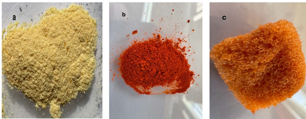
Fig. 1 Photographic images of the synthesized (a) UiO-66-NH 2 , (b) UiO-66-NH-calcein, and (c) PUF/UiO-66-NH-calcein nanocomposite.
