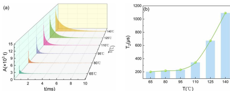
Fig. 2 For F2314 at various temperatures: (a) MSE-FID decays and (b) the corresponding  $T_2$  values.
