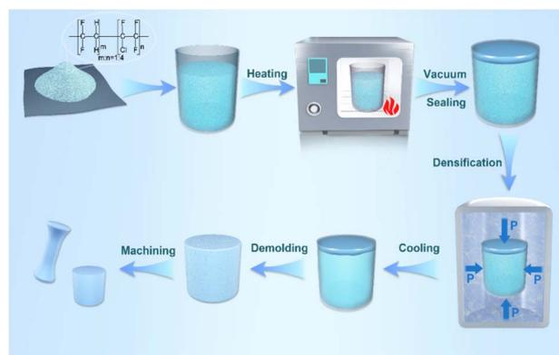
Fig. 1 Schematic illustration of isostatic pressing for F2314.
