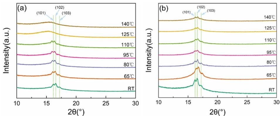
Fig. 7 XRD patterns of F2314 (a) heated and (b) compacted at various temperatures.
