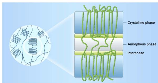
Fig. 3 Schematic depiction of the semicrystalline polymer structure.
