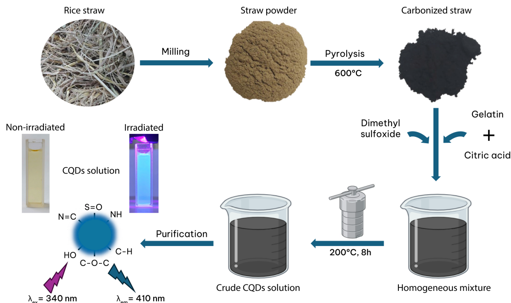
Fig. 1 Synthesis process of nitrogen- and sulfur-co-doped carbon quantum dots (NS-CQDs) from rice straw.
