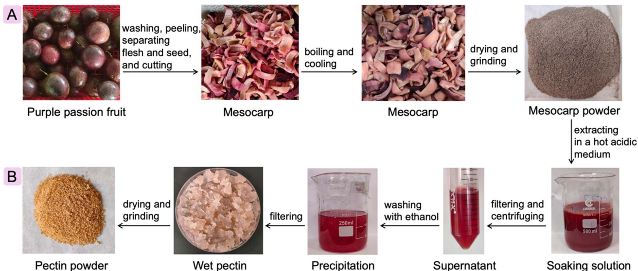
Scheme 1 Process of pre-treatment (A) and the pectin extraction (B) from the passion fruit mesocarp powder.
