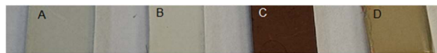
Fig. 2 Photography of as-deposited (A and C) and annealed (B and D) 50 nm TiO 2 layers on FTO support. (A) As-deposited LT-ALD TiO 2 ; (B) annealed LT-ALD TiO 2 ; (C) as-deposited HT-ALD TiO 2 ; (D) annealed HT-ALD TiO 2 .
