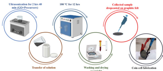
Fig. 1 Schematic for synthesis of BPN n samples followed by symmetric coin cell characterization.
