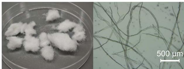
Fig. 3 Macroscopic photograph of bleached softwood kraft pulp board and optical micrographs.
