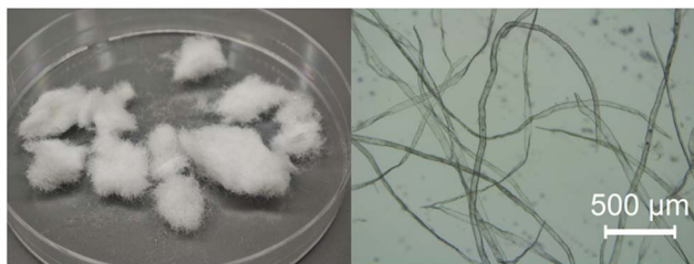
Fig. 3 Macroscopic photograph of bleached softwood kraft pulp board and optical micrographs.
