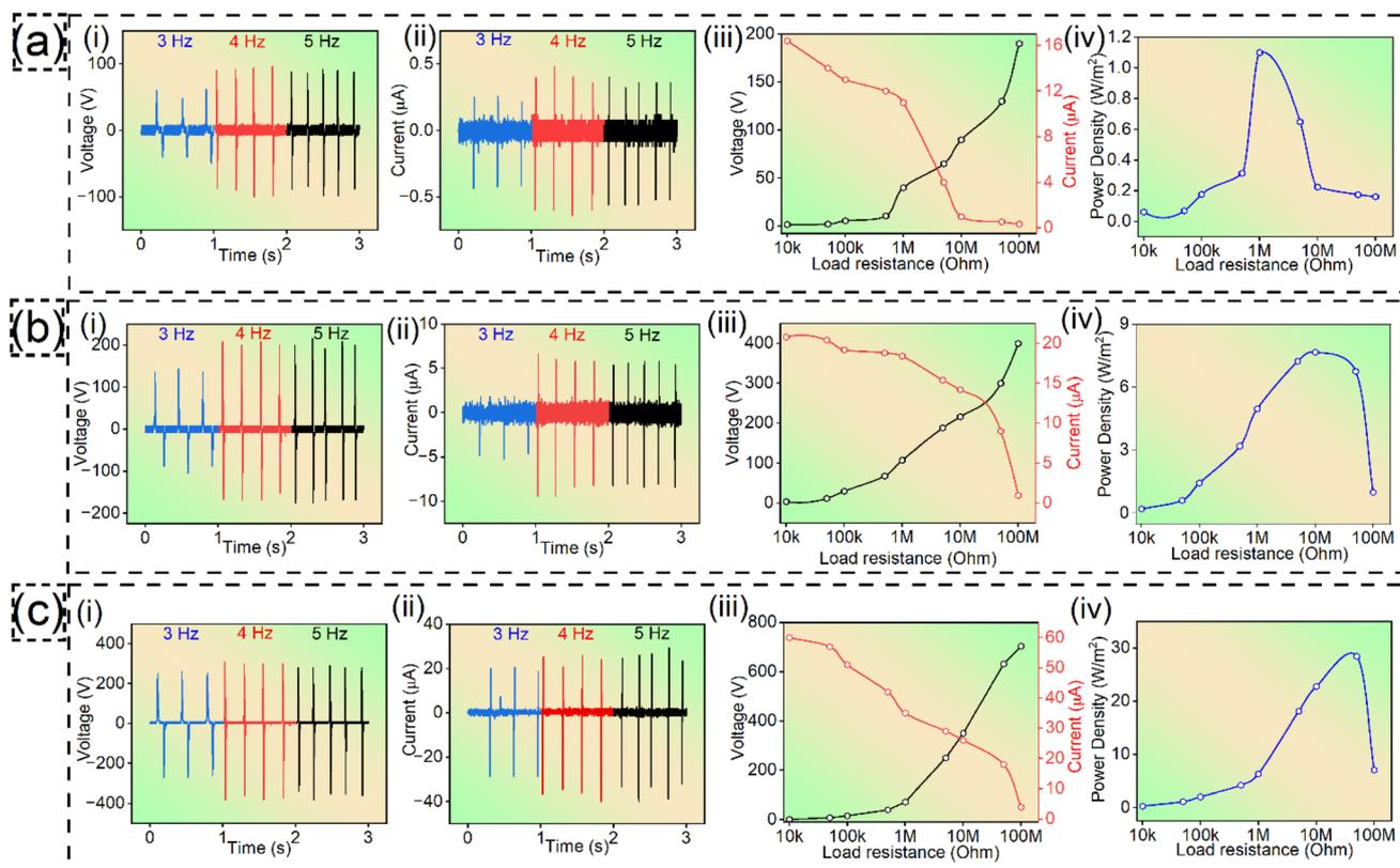
Fig. 5 (i) Open-circuit voltage ( $V_{oc}$ ), (ii) short-circuit current ( $I_{sc}$ ), (iii)  $V_{oc}$  and  $I_{sc}$  with load resistance, and (iv) power-density with load resistance, for (a) SC-PS, (b) ES-PS, and (c) SP-PS, respectively.
