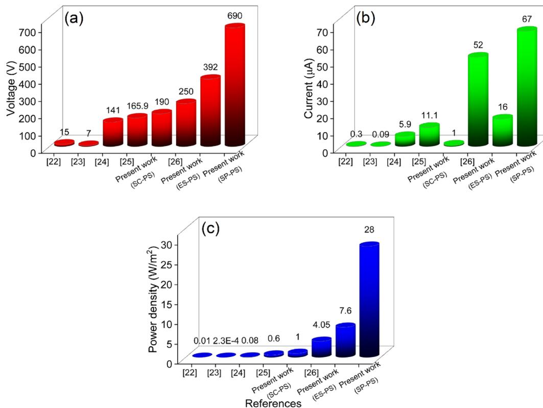
Fig. 6 Triboelectric outputs (a) open-circuit voltage, (b) short-circuit current, and (c) power density reported in the literature<sup>29–33</sup> compared with the present study.
