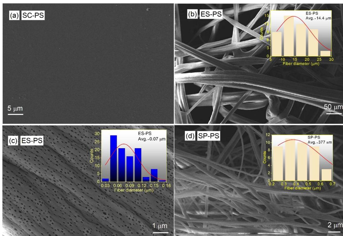
Fig. 3 SEM images of (a) solution casted (SC-PS), (b) and (c) electrospun (ES-PS), and histogram showing fiber analysis and pore size analysis, (d) spray-coated (SP-PS), and histogram showing fiber analysis of synthesized film.
