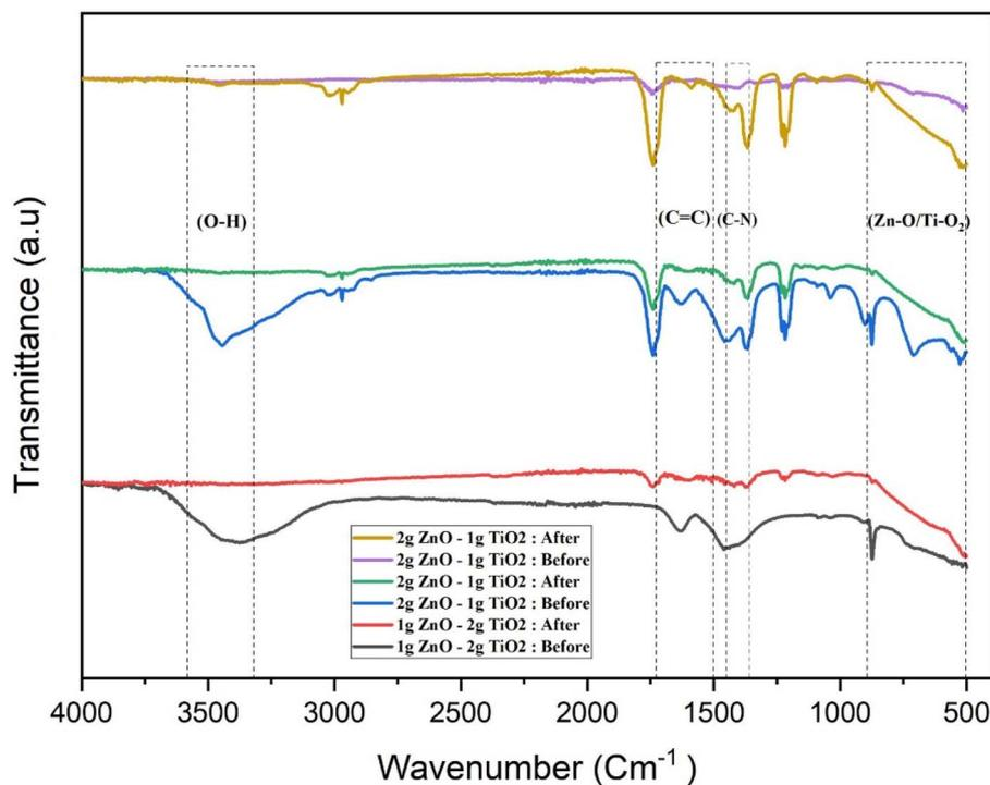
Fig. 3 FTIR spectra of  $\text{TiO}_2/\text{ZnO}$ -CaAlg composites beads before and after CV adsorption.
