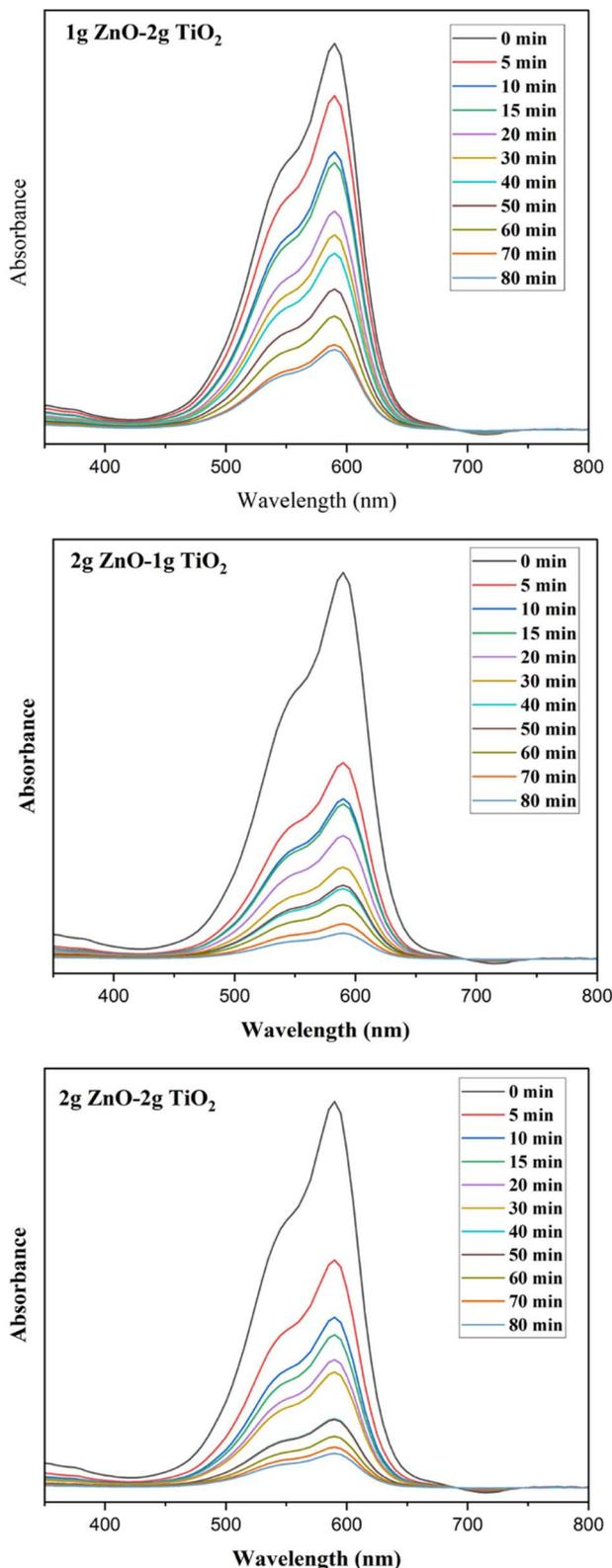
Fig. 6 UV-vis spectral changes of CV solution as a function of degradation time using ZnO/TiO<sub>2</sub>-CaAlg composite beads.
