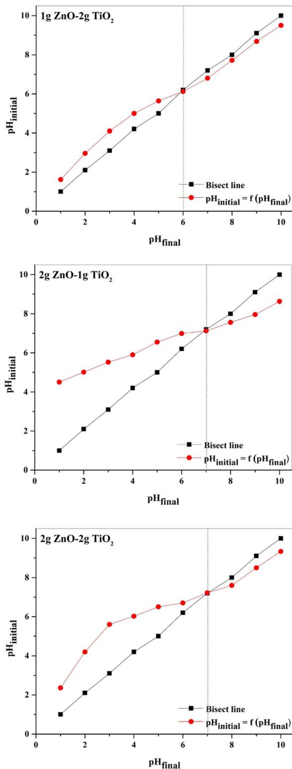
Fig. 7 Zero charge point ( $\text{pH}_{\text{pzc}}$ ) of ZnO/TiO<sub>2</sub>-CaAlg composite beads.
