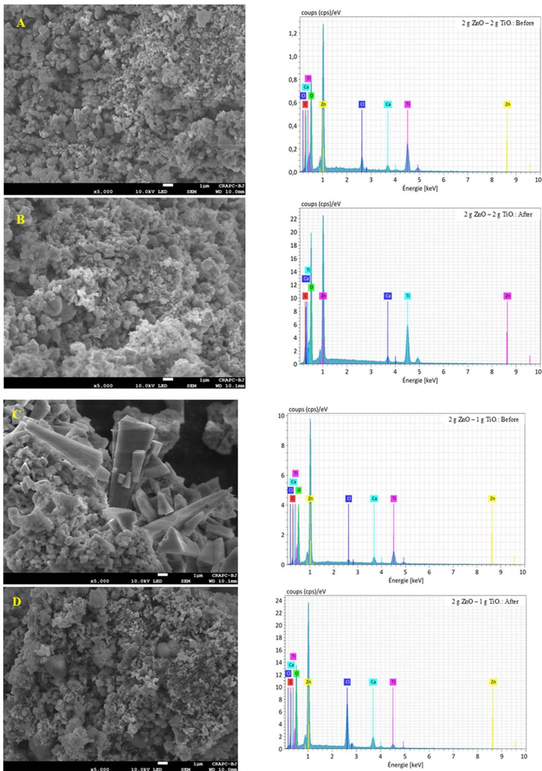
Fig. 5 SEM and EDS analyses of TiO<sub>2</sub>/ZnO–CaAlg composite beads with different TiO<sub>2</sub>/ZnO ratios before and after CV removal: (A) SEM images before adsorption, (B) SEM images after adsorption, (C) EDS spectra before adsorption, and (D) EDS spectra after adsorption.
