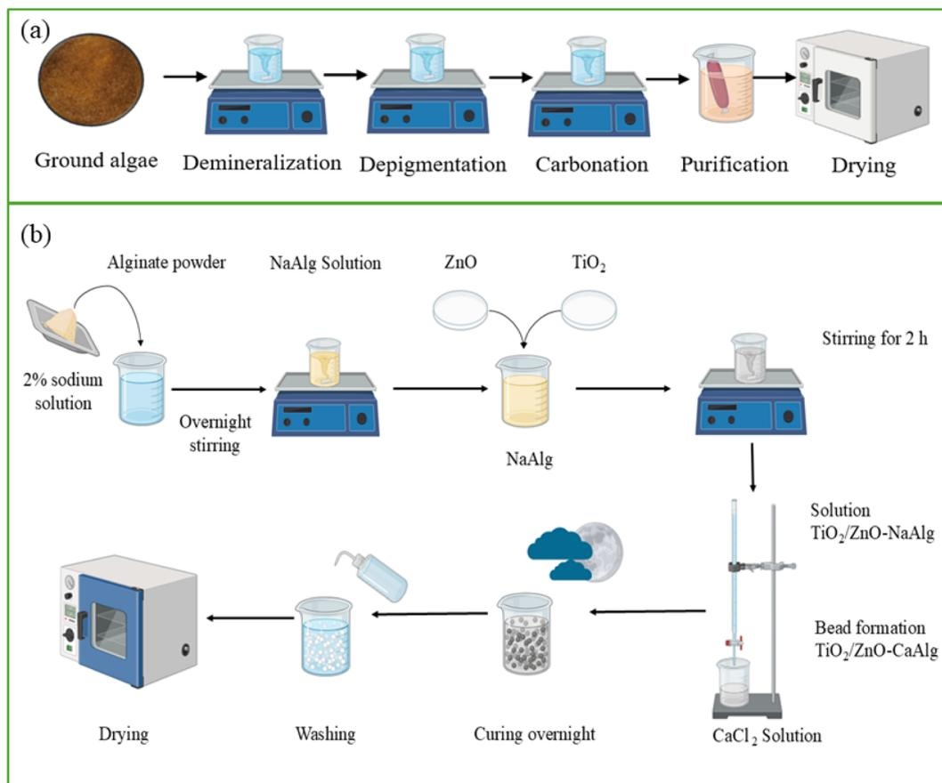
Fig. 2 (a) Schematic illustration of the alginate extraction process; (b) schematic illustration of the TiO<sub>2</sub>/ZnO-CaAlg composite preparation process.
