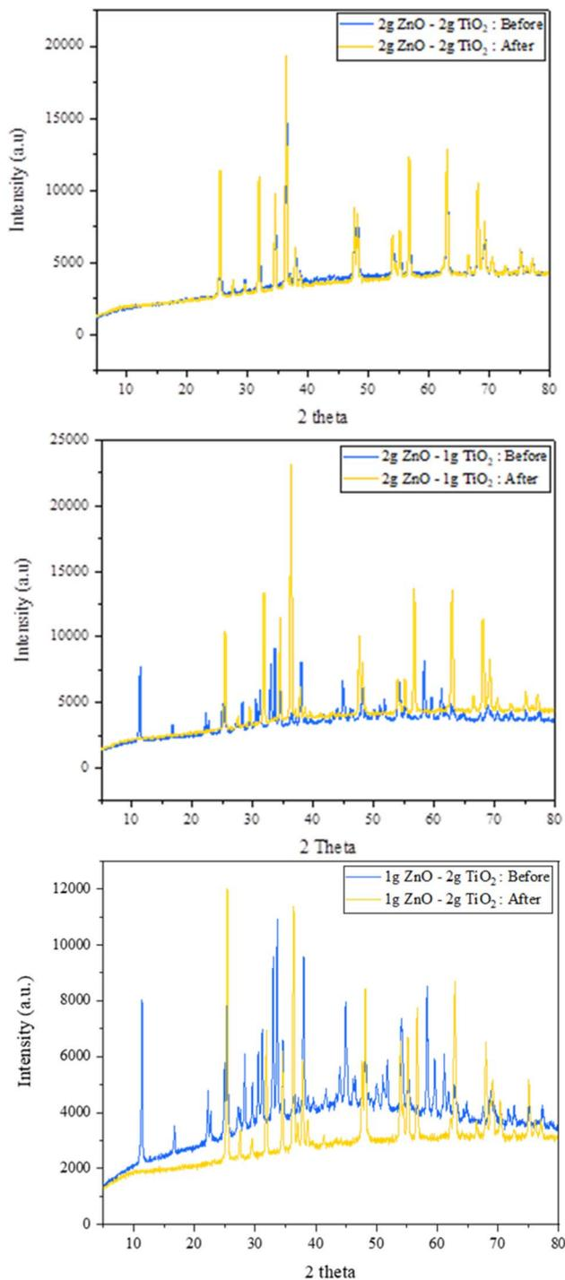
Fig. 4 XRD analysis of  $\text{TiO}_2/\text{ZnO}$ -CaAlg composite beads before and after adsorption and photocatalysis.
