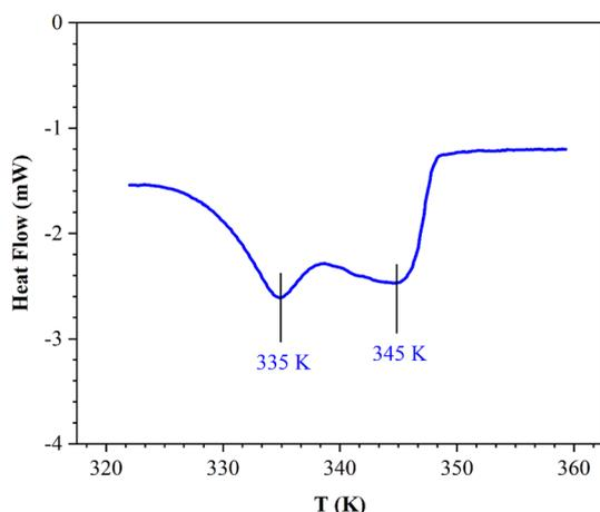
Fig. 7 Differential scattering calorimetric trace of  $[(\text{C}_4\text{H}_9)_4\text{N}]_2\text{CoBr}_4$ .
