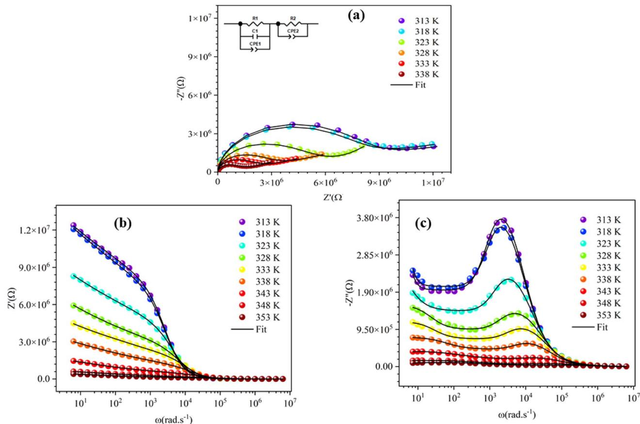
Fig. 8 Complex impedance spectra of  $[\text{N}(\text{C}_4\text{H}_9)_4]_2\text{CoBr}_4$  at different temperatures: (a) complex impedance spectra, (b) variation of the real part  $Z'$  as a function of frequency, and (c) variation of the imaginary part  $Z''$  as a function of frequency.
