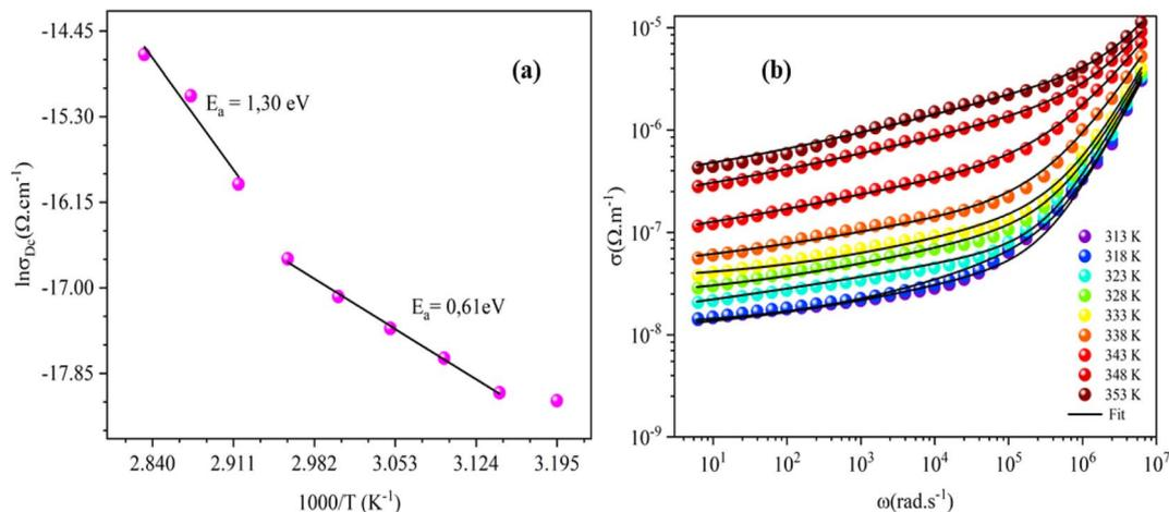
Fig. 9 Temperature dependence of the electrical conductivity of the compound  $[(C_4H_9)_4N]_2CoBr_4$ : (a) variation of  $\ln(\sigma_{DC})$  as a function of  $1000/T$  and (b) evolution of the AC conductivity at different frequencies.
