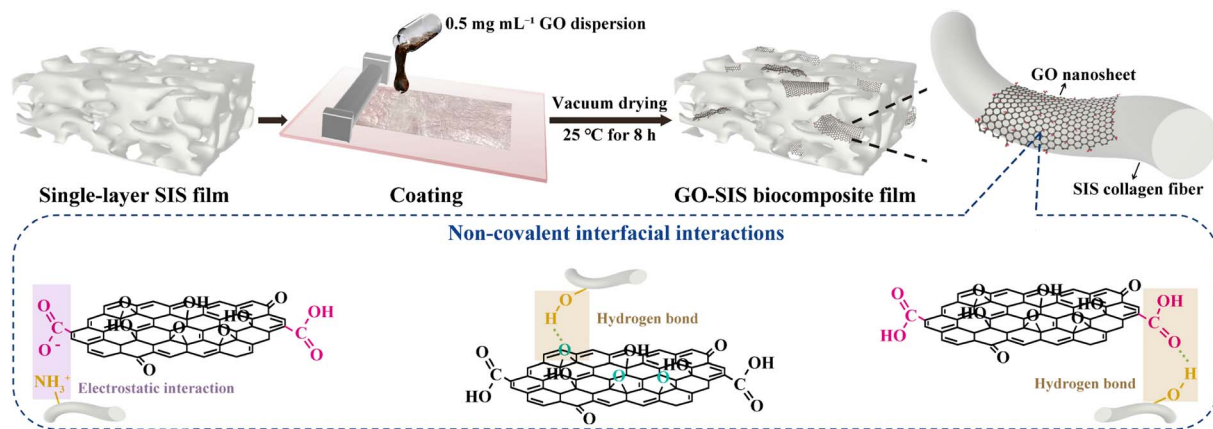
Fig. 1 Schematic of the fabrication process and non-covalent interfacial interactions in the GO-SIS biocomposite film.
