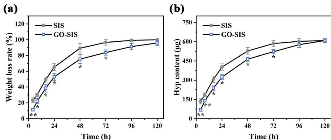
Fig. 9 Quantitative analysis of *in vitro* degradation for SIS and GO-SIS biocomposite films at different time points. (a) Weight loss rate; (b) Hyp content in the degradation solution. Data are presented as mean  $\pm$  standard deviation (SD),  $n = 3$ , \* $p < 0.05$ , \*\* $p < 0.01$ .
