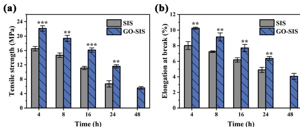
Fig. 10 Mechanical properties of dried SIS and GO-SIS biocomposite films after *in vitro* degradation. (a) Tensile strength, (b) elongation at break. Data are presented as mean  $\pm$  standard deviation (SD),  $n = 3$ , \*\* $p < 0.01$ , \*\*\* $p < 0.001$ .
