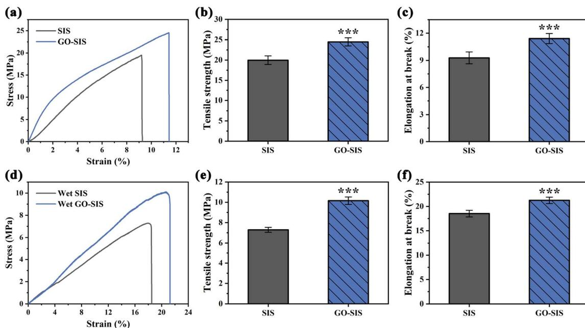
Fig. 6 Mechanical properties of SIS and GO-SIS biocomposite films. (a) Representative stress–strain curves, (b) tensile strength, and (c) elongation at break in the dry state. (d) Representative stress–strain curves, (e) tensile strength, and (f) elongation at break in the wet state. Data are presented as mean  $\pm$  standard deviation (SD),  $n = 5$ ,  $***p < 0.001$ .
