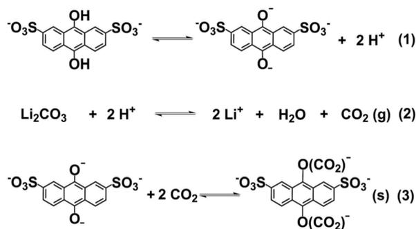
Fig. 4 Reaction equations between AQDSH<sub>2</sub> and CO<sub>2</sub>. The liberated H<sup>+</sup> then reacts with Li<sub>2</sub>CO<sub>3</sub> to release CO<sub>2</sub>, which subsequently combines with AQDS<sup>2-</sup> to form the AQDS(CO<sub>2</sub>)<sub>2</sub><sup>2-</sup> precipitate.
