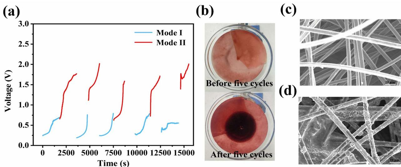
Fig. 5 Cycling Stability. (a) Electrolyzer voltage profiles during five consecutive Mode I/II cycles at 40 mA cm<sup>-2</sup>. (b) The comparison of filtrating solution the in the central compartment before and after five cycles. (c) SEM image of the carbon felt before five cycles. (d) SEM image of the carbon felt after five cycles.
