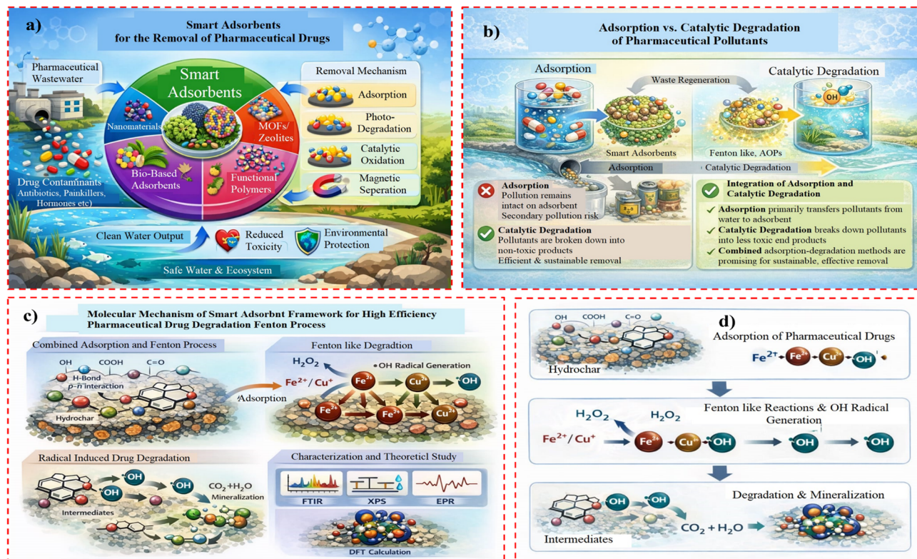
Fig. 2 (a) Conceptual overview of smart adsorbents in pharmaceutical wastewater treatment. (b) From pollutant transfer to pollutant destruction: adsorption and catalytic degradation. (c) Smart adsorbent mechanism for pharmaceutical degradation via the adsorption–Fenton process. (d) Smart adsorbent–Fenton degradation flowchart.
