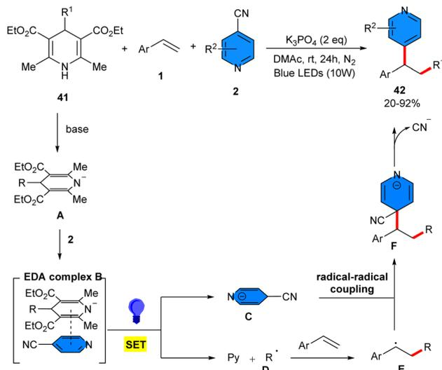
Scheme 25 K<sub>3</sub>PO<sub>4</sub>-mediated alkylarylation of alkenes with 4-cyanopyridines and 4-cyclohexyl-DHP.
