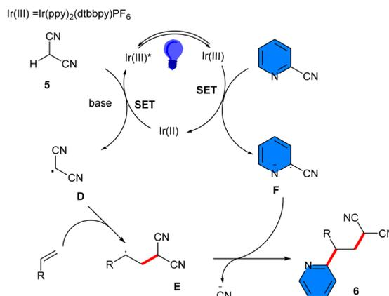
Scheme 2 Plausible mechanism for Ir-catalyzed reaction of alkenes, 4-cyanopyridines, and C(sp<sup>3</sup>)–H feedstocks.
