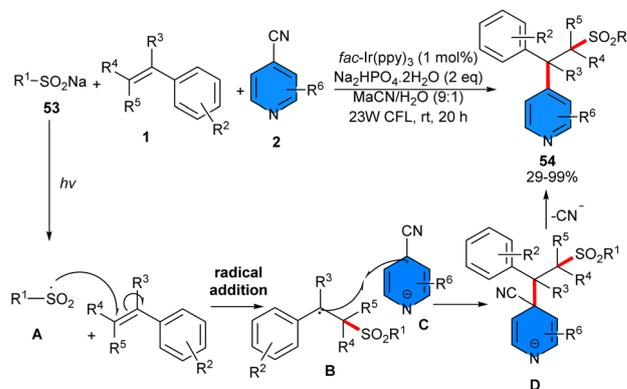
Scheme 33 Ir-catalyzed reaction of styrenes, 4-cyanopyridines and sodium sulfonates.
