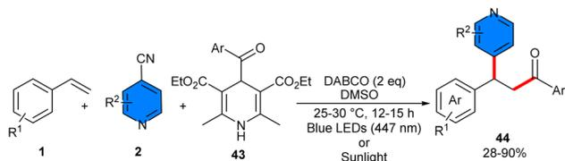
Scheme 26 DABCO-mediated reaction of styrenes, 4-cyanopyridines, and 4-acyl-1,4-dihydropyridines.
