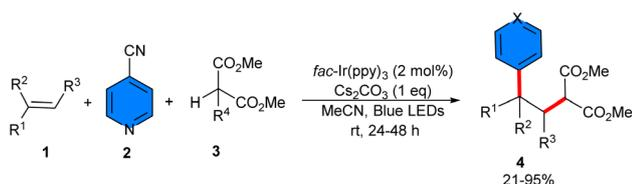
Scheme 1 Ir-catalyzed reaction of alkenes, 4-cyanopyridines, and C(sp<sup>3</sup>)–H feedstocks.
