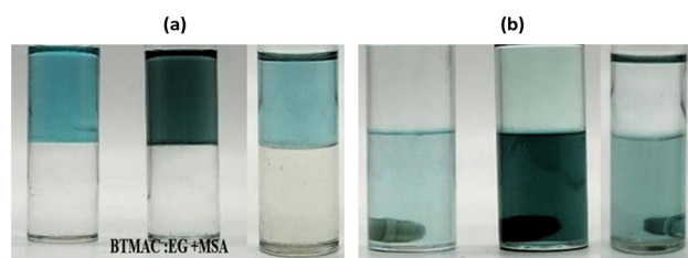
Fig. 3 (a) 0.08 mmol of [\text{Fe}(\text{Pc})] , [\text{Ni}(\text{Pc})] and \text{H}_2\text{Pc} in toluene (top layer) and BTMAC:EG + 10 mmol MSA (bottom layer) before extraction and (b) after extraction for 40 min at 25 °C.
