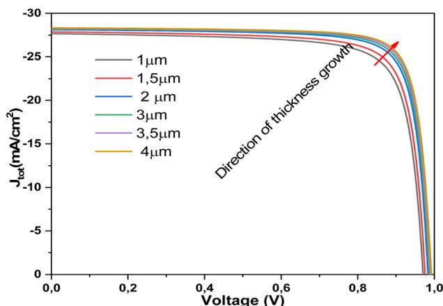
Fig. 2 Current–voltage curves at various absorber thicknesses.
