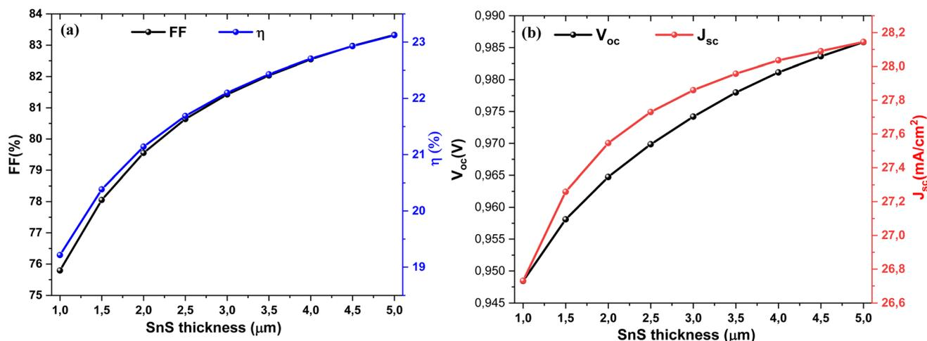
Fig. 3 Dependence of (a) FF and efficiency ( $\eta$ ), and (b)  $V_{oc}$  and  $J_{sc}$  on the SnS layer thickness.
