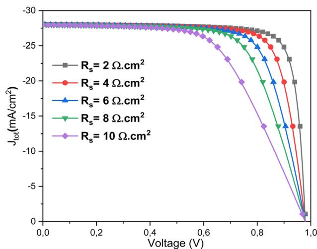
Fig. 15 Current density versus voltage measurements of solar cells at different  $R_s$  values.
