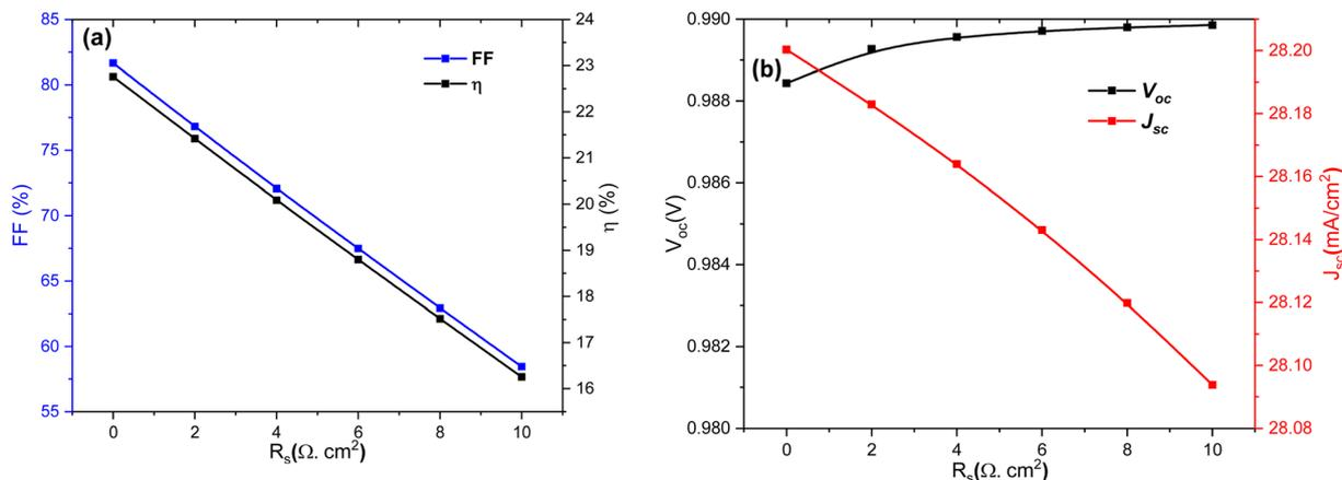
Fig. 16 Dependence of (a) FF and  $\eta$ , and (b)  $V_{oc}$  and  $J_{sc}$  of Al-ZnO/i-ZnO/CdS/SnS solar cells on the  $R_s$ .
