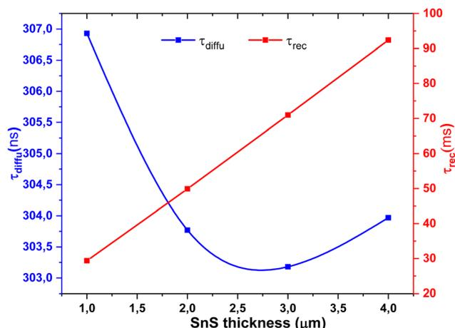
Fig. 14 Variation of relaxation times ( $\tau_{diffu}$  and  $\tau_{rec}$ ) as a function of SnS absorber thickness.
