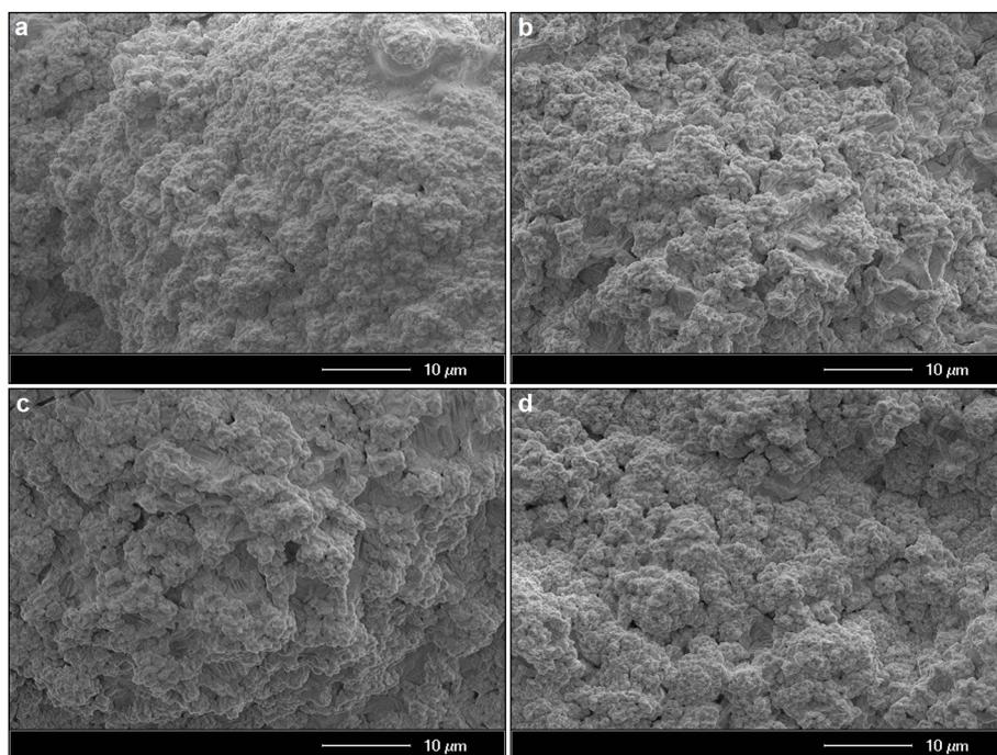
Fig. 4 SEM micrographs of La-based ceramic samples: (a) undoped Ba<sub>2</sub>LaVO<sub>6</sub>, (b) Ba<sub>2</sub>La<sub>0.95</sub>VO<sub>6</sub>:0.05Eu<sup>3+</sup>, (c) Ba<sub>2</sub>La<sub>0.85</sub>VO<sub>6</sub>:0.15Eu<sup>3+</sup>, and (d) Ba<sub>2</sub>La<sub>0.70</sub>VO<sub>6</sub>:0.30Eu<sup>3+</sup>.
