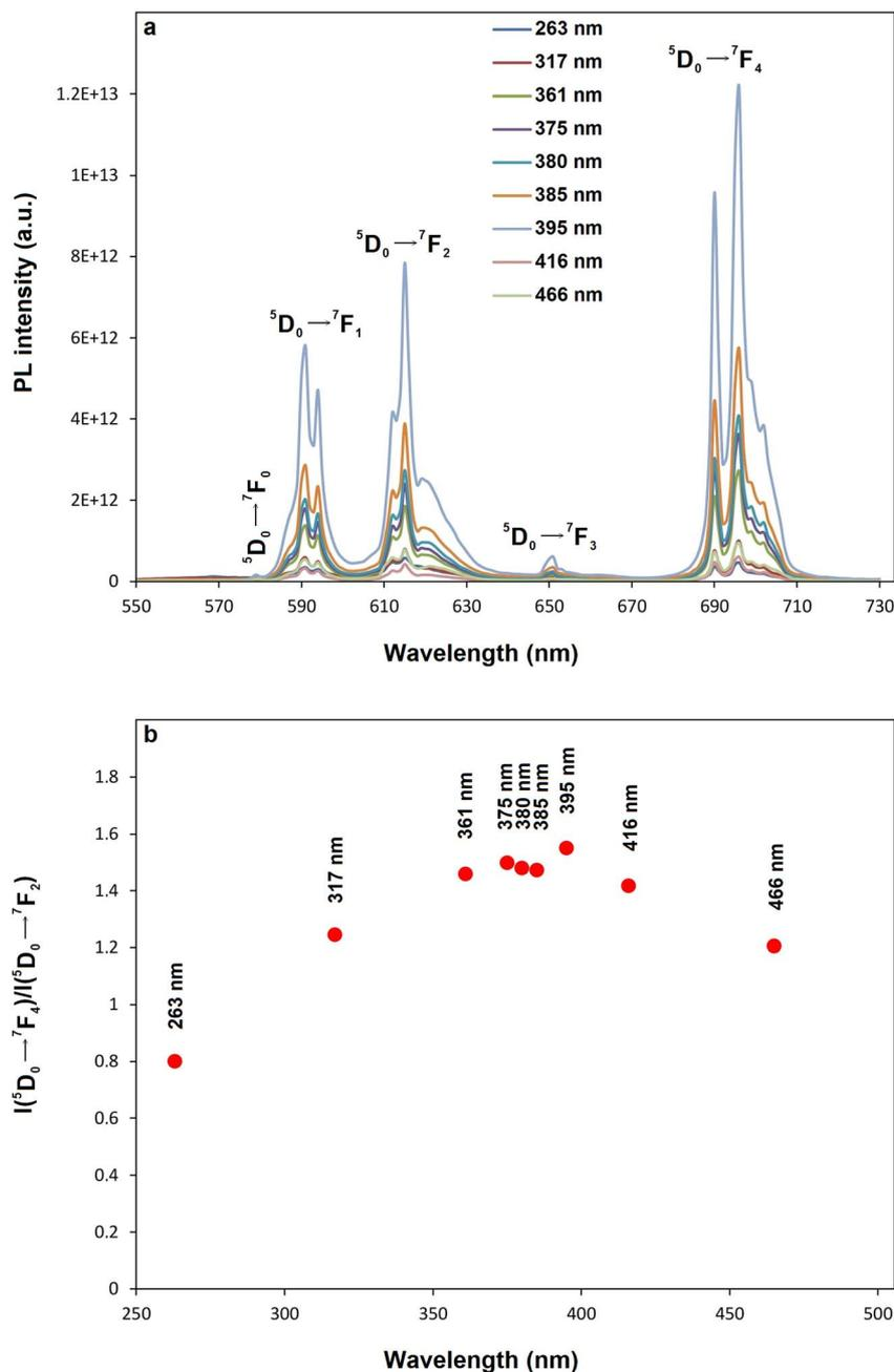
Fig. 8 (a) PL emission spectra of  $\text{Ba}_2\text{LaVO}_6:\text{Eu}^{3+}$  phosphors recorded under different excitation wavelengths, (b) integrated emission intensity of the  ${}^5D_0 \rightarrow {}^7F_4$  transition as a function of excitation wavelength.
