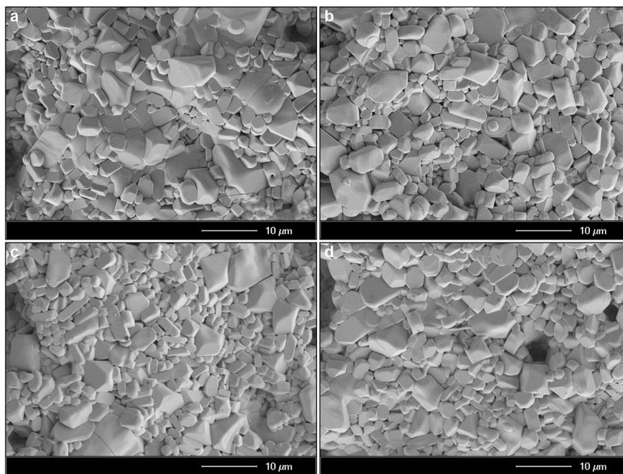
Fig. 5 SEM micrographs of Gd-based ceramic samples: (a) undoped  $\text{Ba}_2\text{GdVO}_6$ , (b)  $\text{Ba}_2\text{Gd}_{0.95}\text{VO}_6:0.05\text{Eu}^{3+}$ , (c)  $\text{Ba}_2\text{Gd}_{0.85}\text{VO}_6:0.15\text{Eu}^{3+}$ , and (d)  $\text{Ba}_2\text{Gd}_{0.70}\text{VO}_6:0.30\text{Eu}^{3+}$ .
