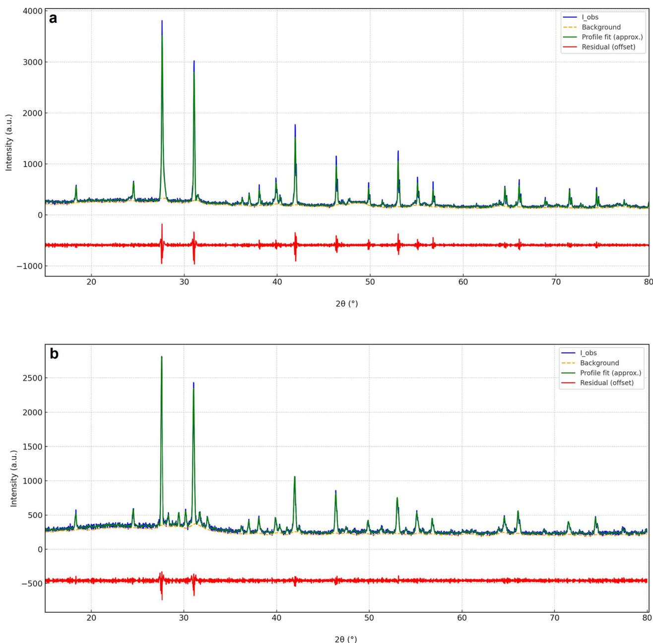
Fig. 3 Rietveld refinement profiles of the undoped double-perovskite hosts refined in the orthorhombic  $Pnma$  space group: (a)  $\text{Ba}_2\text{LaVO}_6$  and (b)  $\text{Ba}_2\text{GdVO}_6$ . Observed, calculated, and difference patterns are shown.
