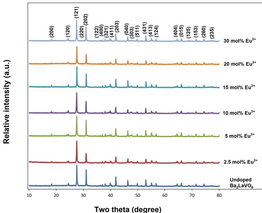
Fig. 1 X-ray diffraction (XRD) patterns of Ba<sub>2</sub>La<sub>1-x</sub>VO<sub>6</sub>:xEu<sup>3+</sup> phosphors with x = 0, 2.5, 5, 10, 15, 20, and 30 mol%, confirming single-phase orthorhombic perovskite formation.
