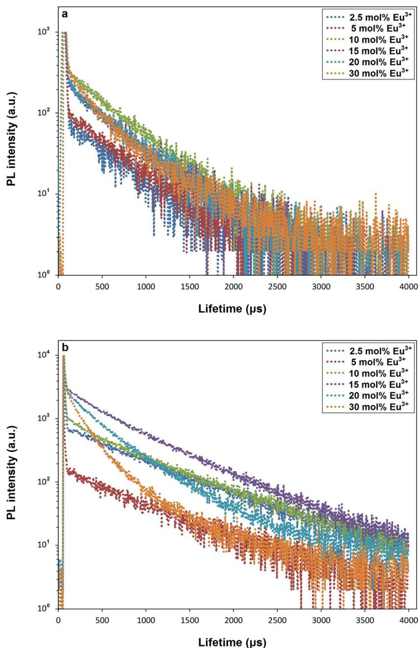
Fig. 9 Luminescence decay curves of (a)  $\text{Ba}_2\text{LaVO}_6:\text{Eu}^{3+}$  and (b)  $\text{Ba}_2\text{GdVO}_6:\text{Eu}^{3+}$  phosphors, excited at 395 and 466 nm and monitored at 696 nm ( $^5\text{D}_0 \rightarrow ^7\text{F}_4$ ) and 611 nm ( $^5\text{D}_0 \rightarrow ^7\text{F}_2$ ), respectively.
