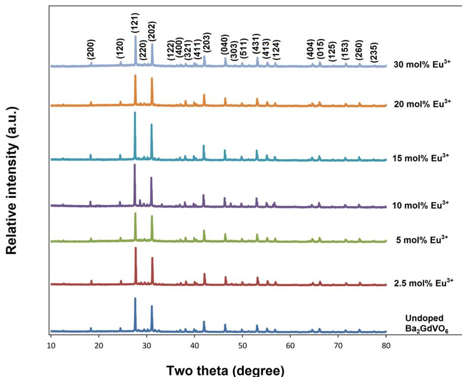
Fig. 2 X-ray diffraction (XRD) patterns of Ba<sub>2</sub>Gd<sub>1-x</sub>VO<sub>6</sub>:xEu<sup>3+</sup> phosphors with x = 0, 2.5, 5, 10, 15, 20, and 30 mol%, indexed to the orthorhombic Pnma structure.
