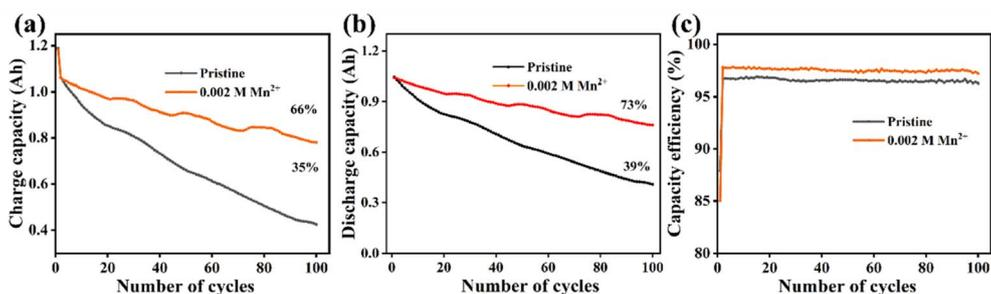
Fig. 7 The cycle performance of ICRFB with and without 0.002 M Mn<sup>2+</sup> anode electrolyte: (a) charge capacity, (b) discharge capacity, and (c) CE.
