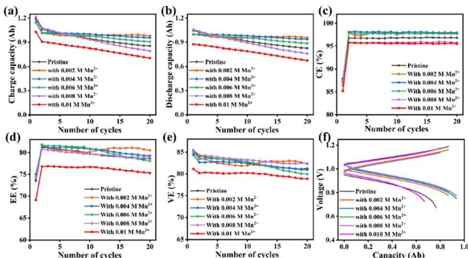
Fig. 3 Effects of concentration of  $\text{Mn}^{2+}$  on ICRFB performance: (a) charge and (b) discharge capacity diagram; (c) CE; (d) EE; (e) VE; (f) capacitance–voltage curve at  $40 \text{ mA cm}^{-2}$ .
