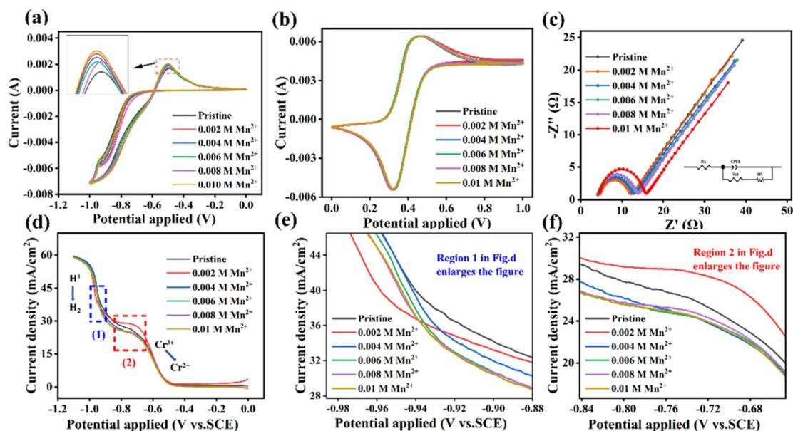
Fig. 4 Effect of  $\text{Mn}^{2+}$  electrolyte on electrochemical behavior: (a) CV curves at a scan rate of  $10 \text{ mV s}^{-1}$  between  $-1$  and  $0 \text{ V}$ ; (b) CV curves at a scan rate of  $10 \text{ mV s}^{-1}$  between  $0$  and  $1 \text{ V}$ ; (c) Nyquist plot at  $0.5 \text{ V}$  and the equivalent circuit diagram; (d) linear sweep voltammetry result; (e) d region 1 enlarged figure; (f) d region 2 enlarged figure.
