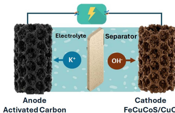
Fig. 2 Asymmetric supercapacitor device of Fe 0.67 Cu 0.22 Co 0.11 S/CuO vs. activated carbon (AC).
