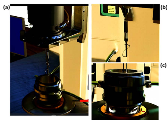
Fig. 1 Presentation of (a) the rheo-reactor system, (b) the static stirring device (torque captor), and (c) the cylindrical tank (shear generator).
