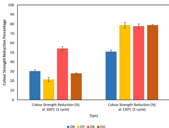
Fig. 5 Percentage reduction in colour strength of dyed polyester fabrics following dye removal at 100 °C and 130 °C. Common treatment conditions included a C : W ratio of 75 : 25, a treatment duration of 30 minutes, and a fabric loading of 10%.
