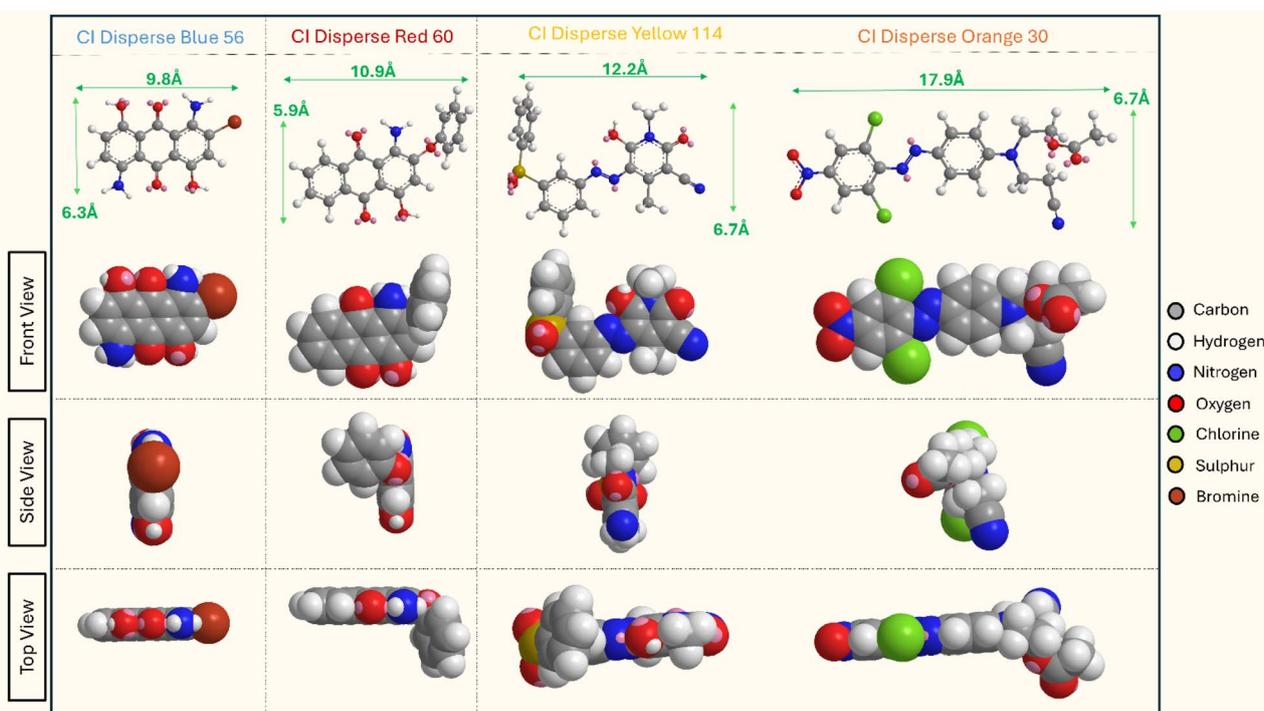
Fig. 8 Modelled 3d structures of four disperse dyes.
