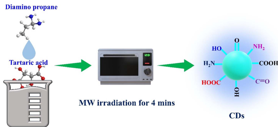
Fig. 1 Microwave-assisted synthesis outline of CDs.
