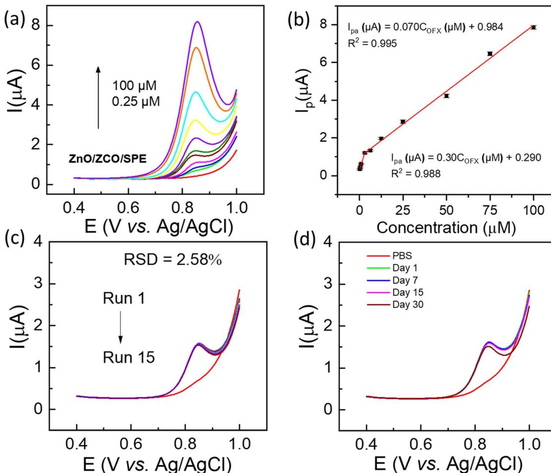
Fig. 7 (a) DPV curves recorded on the SPE electrode modified by ZnO/ZnCo<sub>2</sub>O<sub>4</sub> heterostructures in 0.1 M PBS (pH = 4.0) containing different concentrations of OFL; (b) the corresponding calibration plot of  $I_{pa}$  and  $C_{OFL}$  with error bars; (c) DPV tests of 5  $\mu$ M OFL with 15 consecutive runs in 0.1 M PBS (pH = 4.0); (d) stability tests of ZnO/ZCO/SPE electrode.
