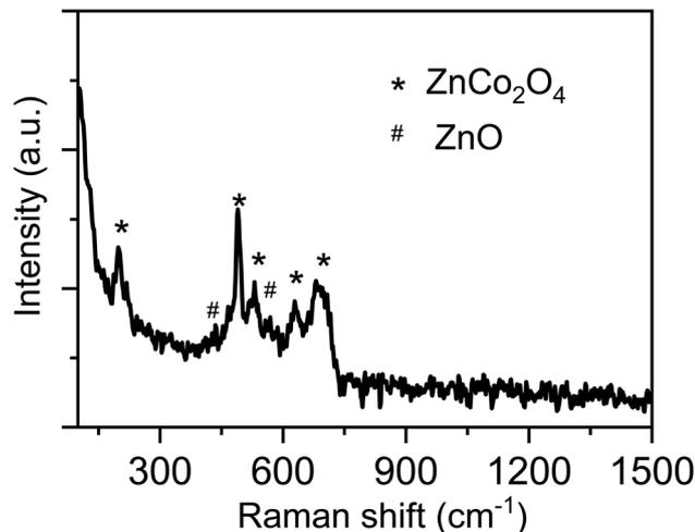
Fig. 2 Raman spectrum of ZnO/ZnCo<sub>2</sub>O<sub>4</sub> heterostructures.
