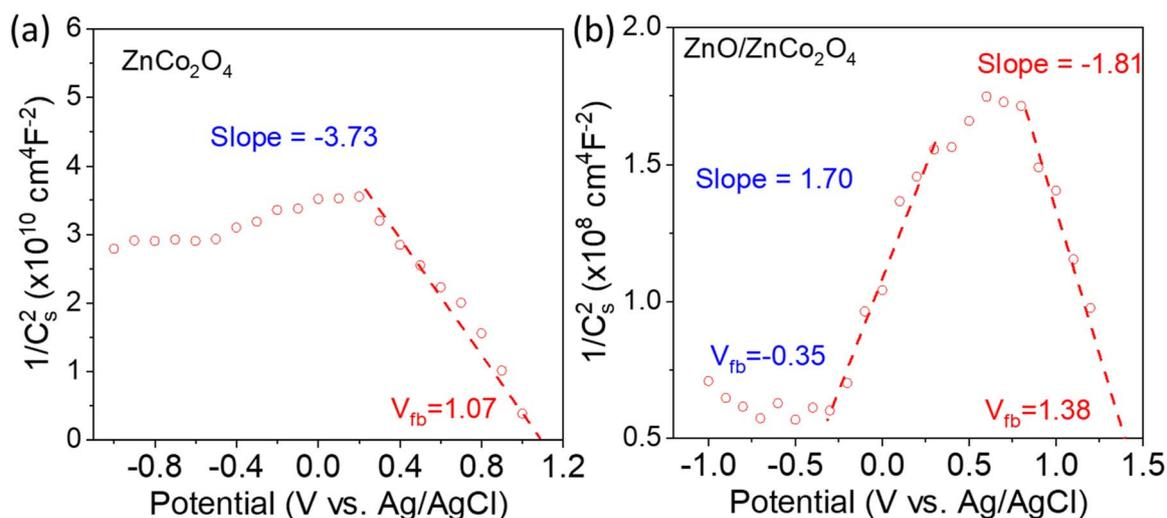
Fig. 3 The Mott–schottky plots of (a) ZnCo<sub>2</sub>O<sub>4</sub> and (b) ZnO/ZnCo<sub>2</sub>O<sub>4</sub> in 0.1 M Na<sub>2</sub>SO<sub>4</sub>.
