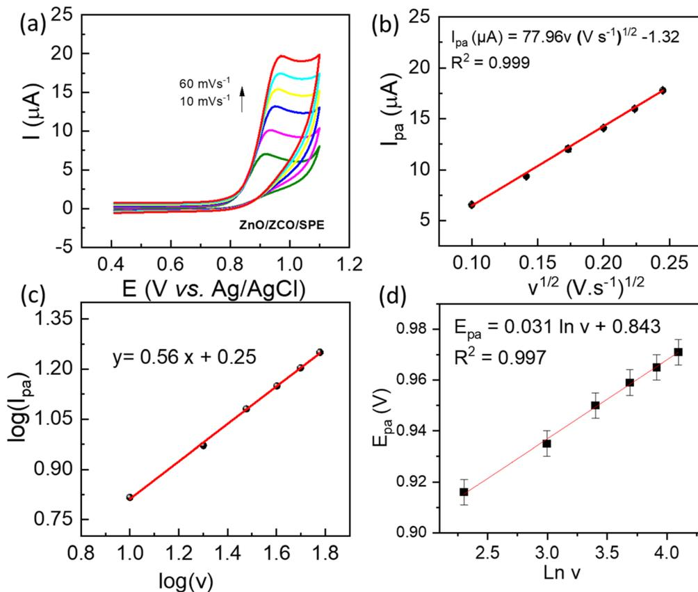
Fig. 5 (a) CV responses of 100  $\mu\text{M}$  OFL on ZnO/ZCO/SPE in 0.1 M PBS (pH = 7.0) with different scan rates ranging from 10  $\text{mV s}^{-1}$  to 60  $\text{mV s}^{-1}$ , the corresponding calibration plots of (b)  $I_{\text{pa}}$  vs.  $v^{1/2}$ ; (c)  $\log(I_{\text{pa}})$  vs.  $\log(v)$ ; and (d)  $E_{\text{pa}}$  vs.  $\ln(v)$ .
