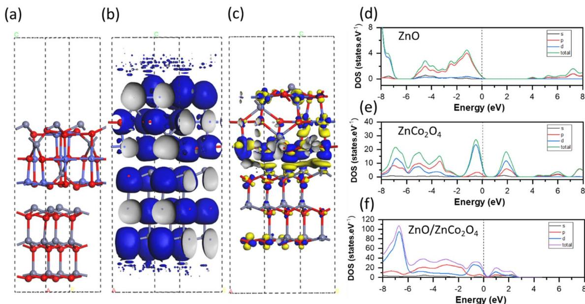
Fig. 8 (a) Lattice structure, (b) electron localization function, (c) iso-surface electron density differences (yellow: electron depletion and blue: electron accumulation) of the ZnO (001)/ZnCo<sub>2</sub>O<sub>4</sub> (001) heterostructure, (d–f) the DOS of calculation of ZnO, ZnCo<sub>2</sub>O<sub>4</sub>, and ZnO/ZnCo<sub>2</sub>O<sub>4</sub> heterostructures.
