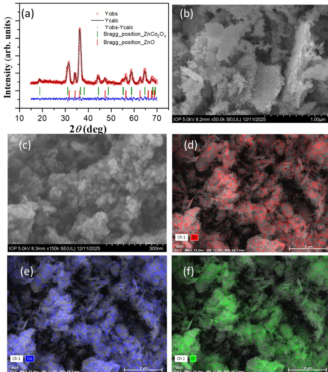
Fig. 1 (a) X-ray, (b and c) FE-SEM, and (d–f) EDX elemental mapping images of ZnO/ZnCo<sub>2</sub>O<sub>4</sub> heterostructures.
