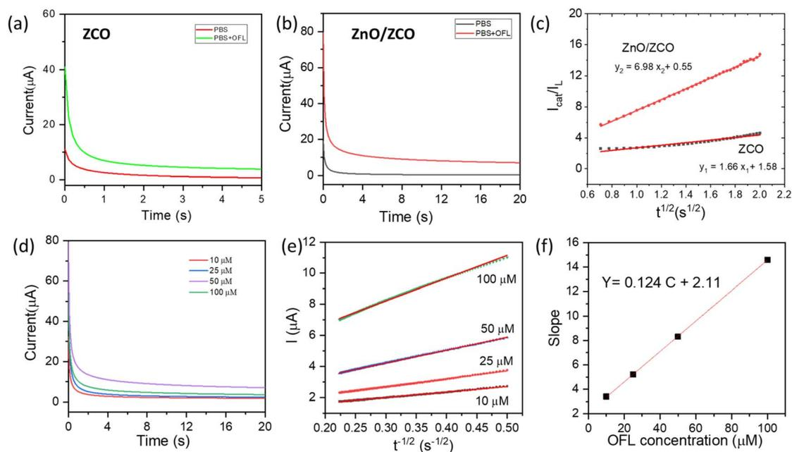
Fig. 6 Chronoamperograms for (a) ZCO/SPE and (b) ZnO/ZnCo<sub>2</sub>O<sub>4</sub>/SPE (20 s) in the absence and presence of 100  $\mu\text{M}$  OFL, and (c) corresponding calibration plots of  $I_{\text{cat}}/I_{\text{L}}$  vs.  $t^{1/2}$ , (d) chronoamperograms for ZnO/ZCO/SPE in the presence of various OFL concentrations, (e) corresponding calibration plots of  $I$  vs.  $t^{1/2}$ , (f) corresponding calibration plots of slope vs. OFL concentration.
