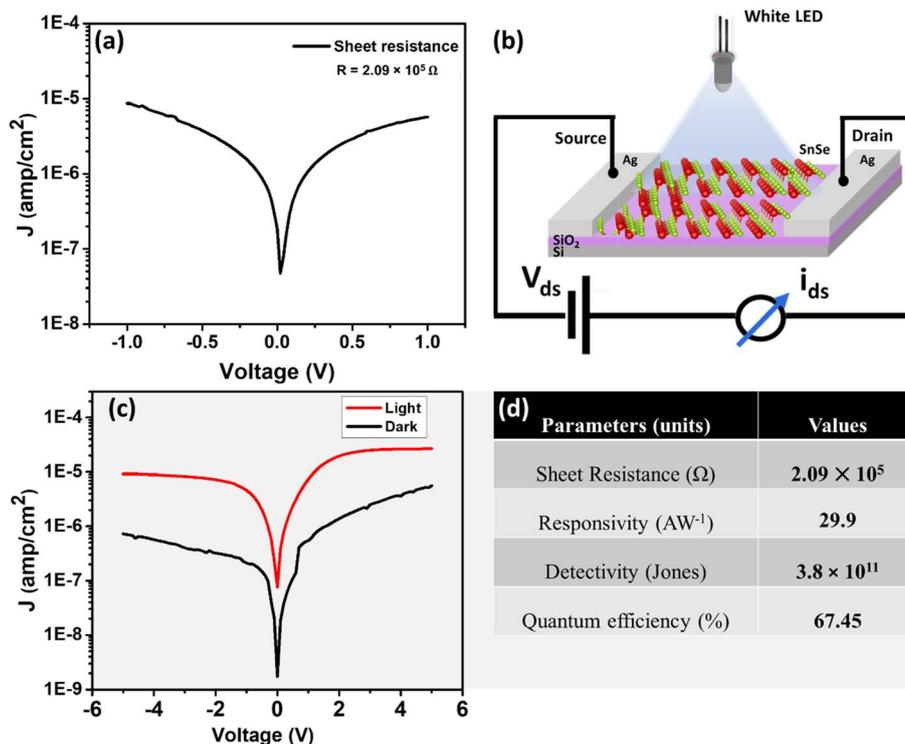
Fig. 5 (a)  $I$ - $V$  characteristics of the SnSe thin film under ambient conditions, enabling calculation of sheet resistance. (b) Schematic representation of the two-probe photoresponse measurement setup under white LED illumination (550 nm). (c)  $I$ - $V$  curves under dark and illuminated conditions showing enhanced current under light exposure due to photogenerated carriers. (d) Summary of extracted photodetector parameters including responsivity, detectivity, and quantum efficiency.
