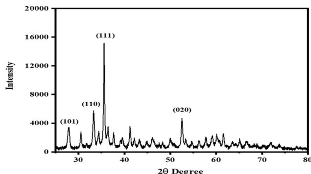
Fig. 3 XRD pattern of synthesized CuO NPs with different peaks.
