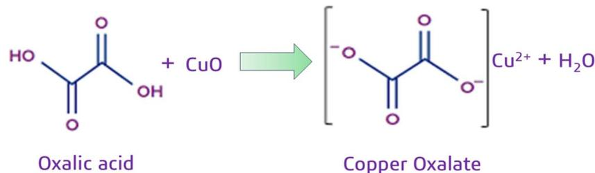
**Scheme 1** Detection of oxalate with CuO NPs utilizing their intrinsic properties. The blue CuO NPs undergo a chemical reaction after incorporation of oxalic acid, forming copper oxalate. This reaction causes a striking blue-to-colorless transition, which can then be precisely used to measure the amount of oxalic acid present in various samples.
