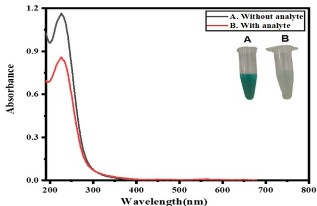
Fig. 6 UV-visible spectrum of CuO NPs. A: CuO NPs without the addition of oxalate solution have high absorbance. B: CuO NPs with the addition of oxalate have low absorbance.
