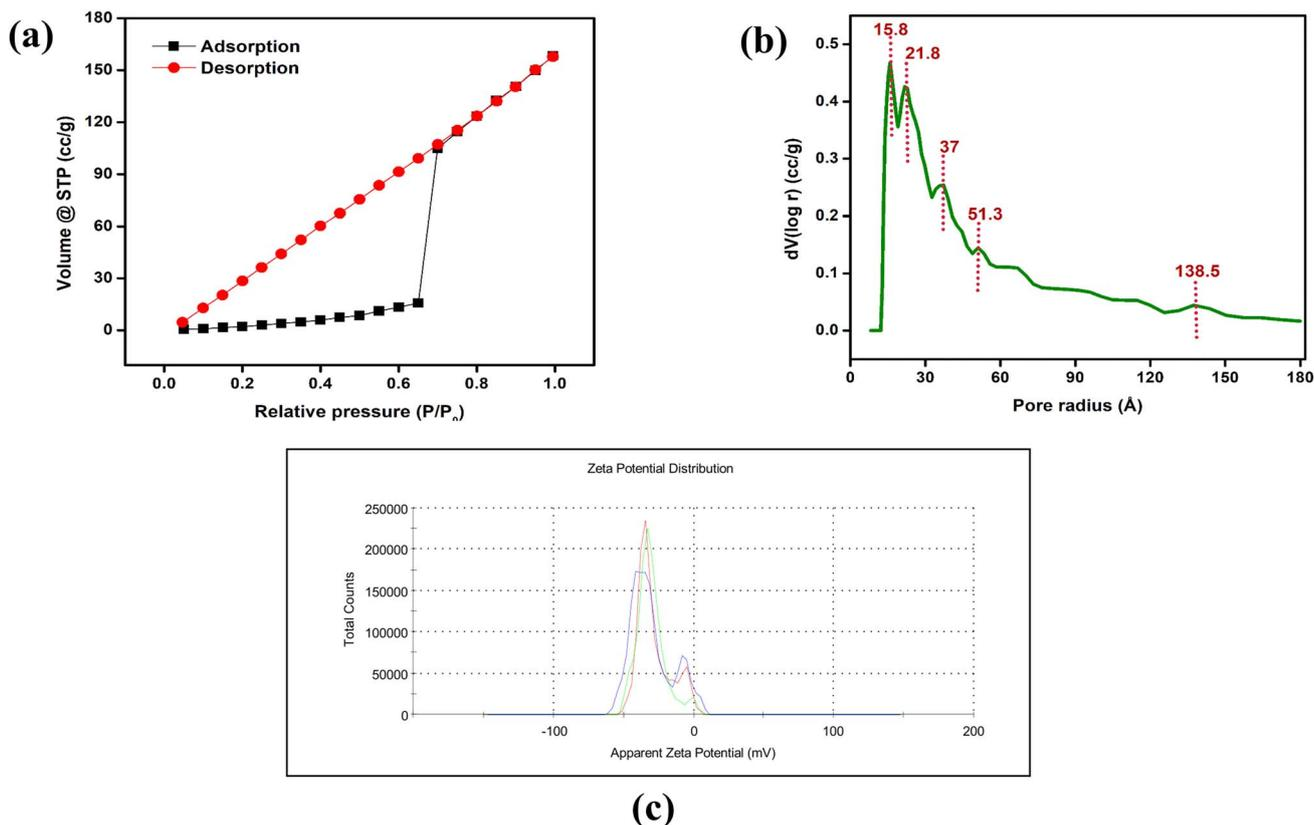
Fig. 6 (a) N<sub>2</sub> adsorption–desorption isotherm curve, (b) distribution graphs of pore size, and (c) zeta Potential.
