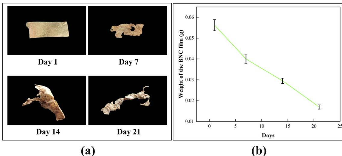
Fig. 13 (a) Morphological changes of BNC film during 21 days of soil burial and (b) changes in weight during 21 days.
