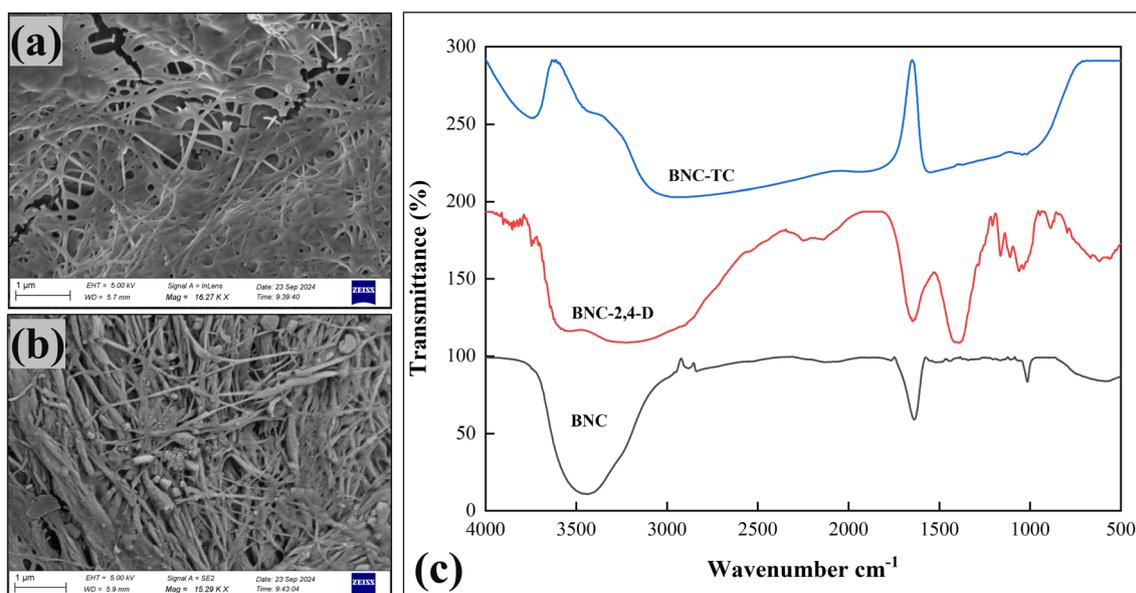
Fig. 8 FE-SEM images of the BNC post-adsorption of (a) TC (magnification = 16.27 kX; scale bar =  $1 \mu\text{m}$ ), (b) 2,4-D (magnification = 15.29 kX; scale bar =  $1 \mu\text{m}$ ), and (c) FTIR spectrum of pre- and post-adsorption of TC and 2,4-D.
