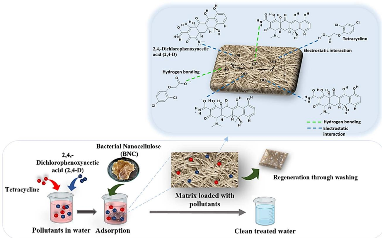
Fig. 7 Adsorption mechanism of the pollutants onto BNC.
