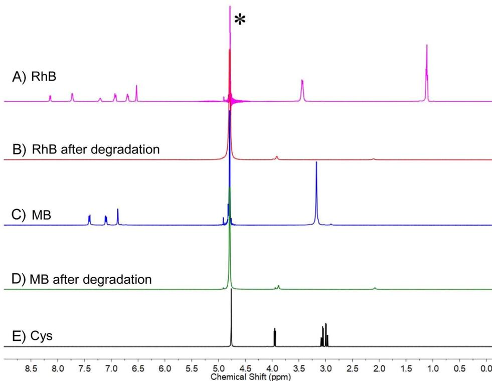
Fig. 3 <sup>1</sup>H-NMR spectra of (A) pure RhB (pink), (B) RhB after degradation in the presence of Cys-Cu NC and H<sub>2</sub>O<sub>2</sub> (red), (C) pure MB (blue), (D) MB after degradation in the presence of Cys-Cu NC and H<sub>2</sub>O<sub>2</sub> (green), and (E) pure Cys (black). The strong solvent peak of D<sub>2</sub>O observed at 4.79 ppm is denoted by an asterisk (\*).
