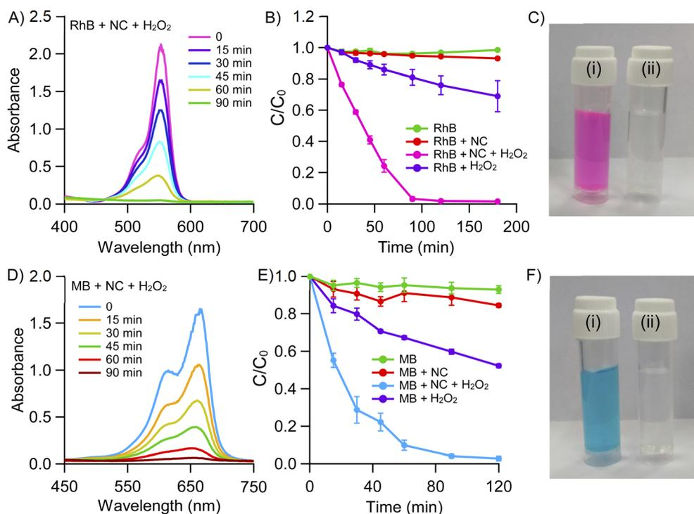
Fig. 1 Cys-Cu NC-mediated degradation of (A–C) RhB and (D–F) MB: time-dependent absorption spectra of (A) RhB and (D) MB with Cys-Cu NC +  $\text{H}_2\text{O}_2$ . Degradation profiles ( $C/C_0$  vs. time) of (B) RhB and (E) MB with Cys-Cu NC +  $\text{H}_2\text{O}_2$  and with different controls. Solution colour changes of (C) RhB and (F) MB (i) before and (ii) after degradation.
