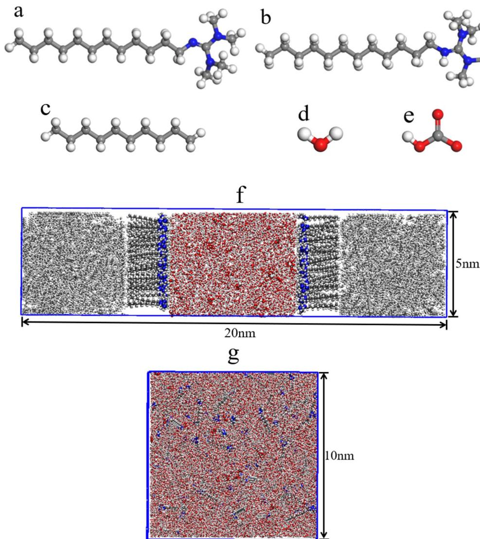
Fig. 1 (a)–(e) Structures of DTMG, DTMGH, *n*-decane, water, and bicarbonate ion. (f) Initial configuration of the surfactant oil–water interface model, (g) initial configuration of the surfactant emulsification model. Grey represents carbon atoms, white represents hydrogen atoms, red represents oxygen atoms, and blue represents nitrogen atoms.
