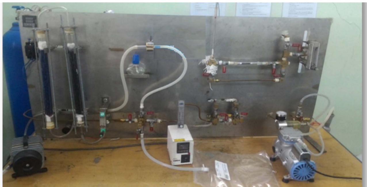
Fig. 2 Schematic representation and photograph of the laboratory-scale batch-wise gas adsorption system for BTEX adsorption. Symbols: 1 – delivery pump; 2 – AC-packed column; 3 – rubber stopper; 4 – glass wool plug; 5 – silica gel-packed column; 6 – coiled copper tube; 7 – fixed-bed adsorption column; 8 – vacuum pump; 9 – alcohol lamp; 10 – alignment point; 11 – glass evaporation chamber; 12 – heating chamber with plate heater; 13 – liquid BTEX droplet; 14 – spent adsorption column; 15 – Tedlar gas sampling bag; V1–V15 – brass gas valves; F1–F3 – mass flow controller; TCU – temperature control unit; T – temperature sensor.
