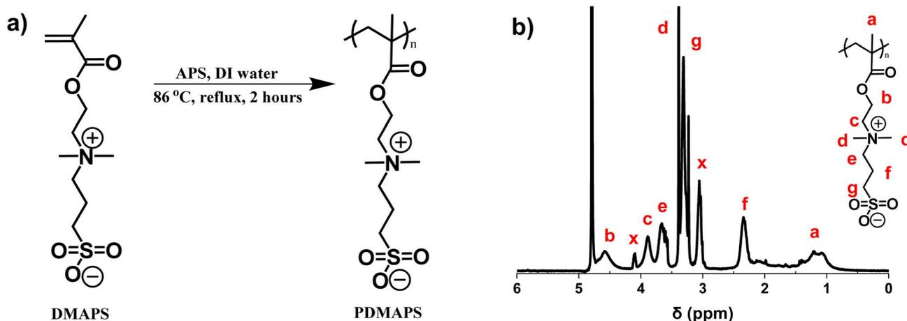
Fig. 1 Synthesis of PDMAPS by FRP of DMAPS, initiated with APS in water (a); <sup>1</sup>H-NMR spectrum in D<sub>2</sub>O containing 0.5 M NaCl at 25 °C (b). Conditions for FRP: DMAPS/water = 0.4/1 (e.g., 40 wt% DMAPS over water); 0.5 wt% of APS over DMAPS.
