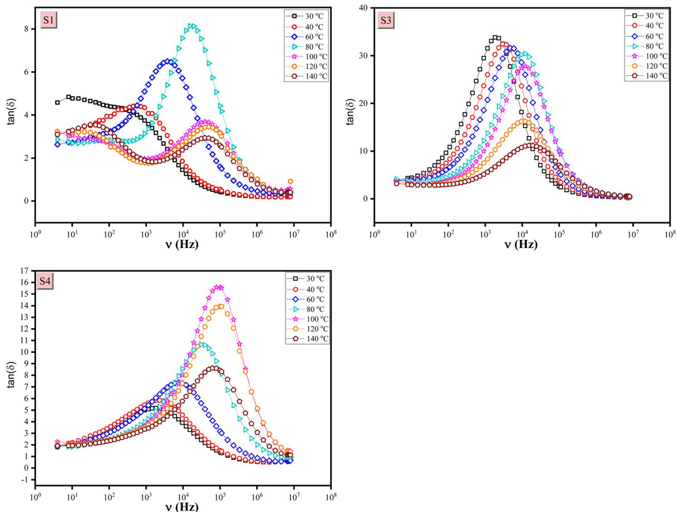
Fig. 6 Loss tangent ( $\tan(\delta)$ ) of HEC and HEC@ZnCe<sub>0.3</sub>Ti<sub>0.7</sub>O<sub>3</sub> nanocomposites (S1, S3, and S4) at different temperatures (30 to 140 °C).
