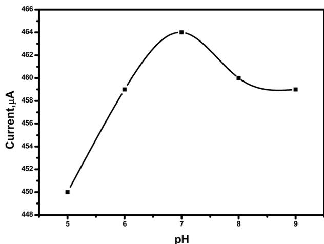
Fig. 13 pH effect of PBS buffer on the chronoamperometry peaks current of peroxide oxidation using the HEC and HEC@ZnCe<sub>0.3</sub>Ti<sub>0.7</sub>O<sub>3</sub> nanocomposites modified SPEs.
