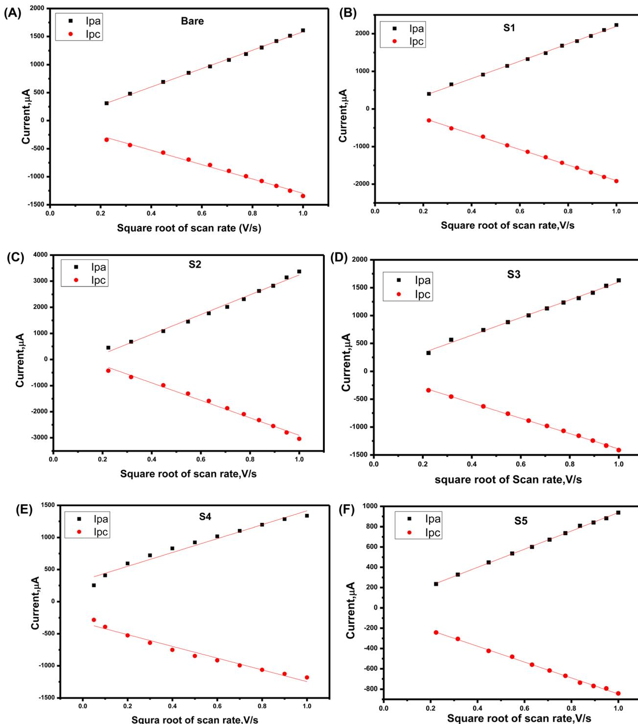
Fig. 11 Anodic ( $I_{pa}$ ) and cathodic ( $I_{pc}$ ) peak currents vs. the square root of the scan rate of (A) bare, (B) S1 (C) S2, (D) S3 (E) S4, and (F) S5 modified screen printed electrodes using a solution containing 5 mM ferro/ferricyanide and 0.1 M KCl.
