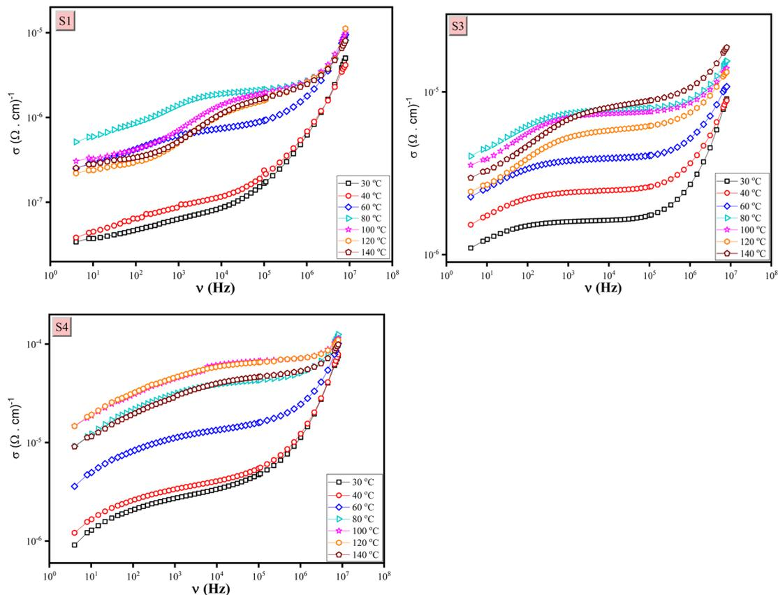
Fig. 8 AC conductivity ( $\sigma$ ) of HEC and HEC@ZnCe<sub>0.3</sub>Ti<sub>0.7</sub>O<sub>3</sub> nanocomposites (S1, S3, and S4) at different temperatures (30 to 140 °C).
