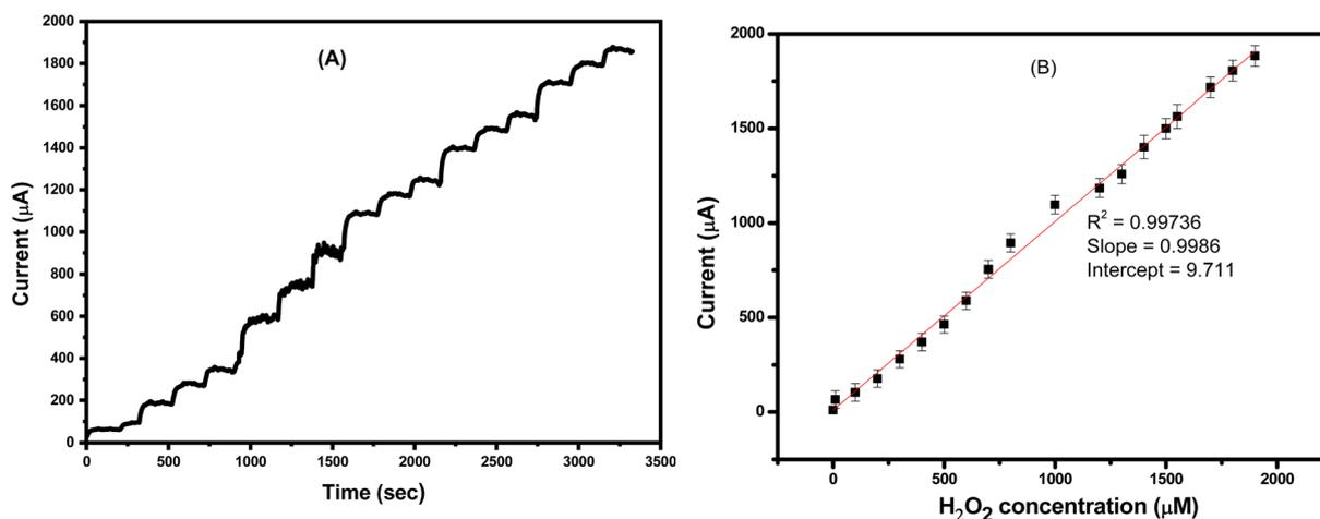
Fig. 14 (A) Chronoamperometric (CA) responses recorded at a fixed potential of 0.7 V, and (B) the corresponding linear calibration curve of current versus H<sub>2</sub>O<sub>2</sub> concentration with R<sup>2</sup> = 0.997. The measurements were performed using the S2 electrode after successive additions of various H<sub>2</sub>O<sub>2</sub> concentrations in PBS buffer (pH 7.0).
