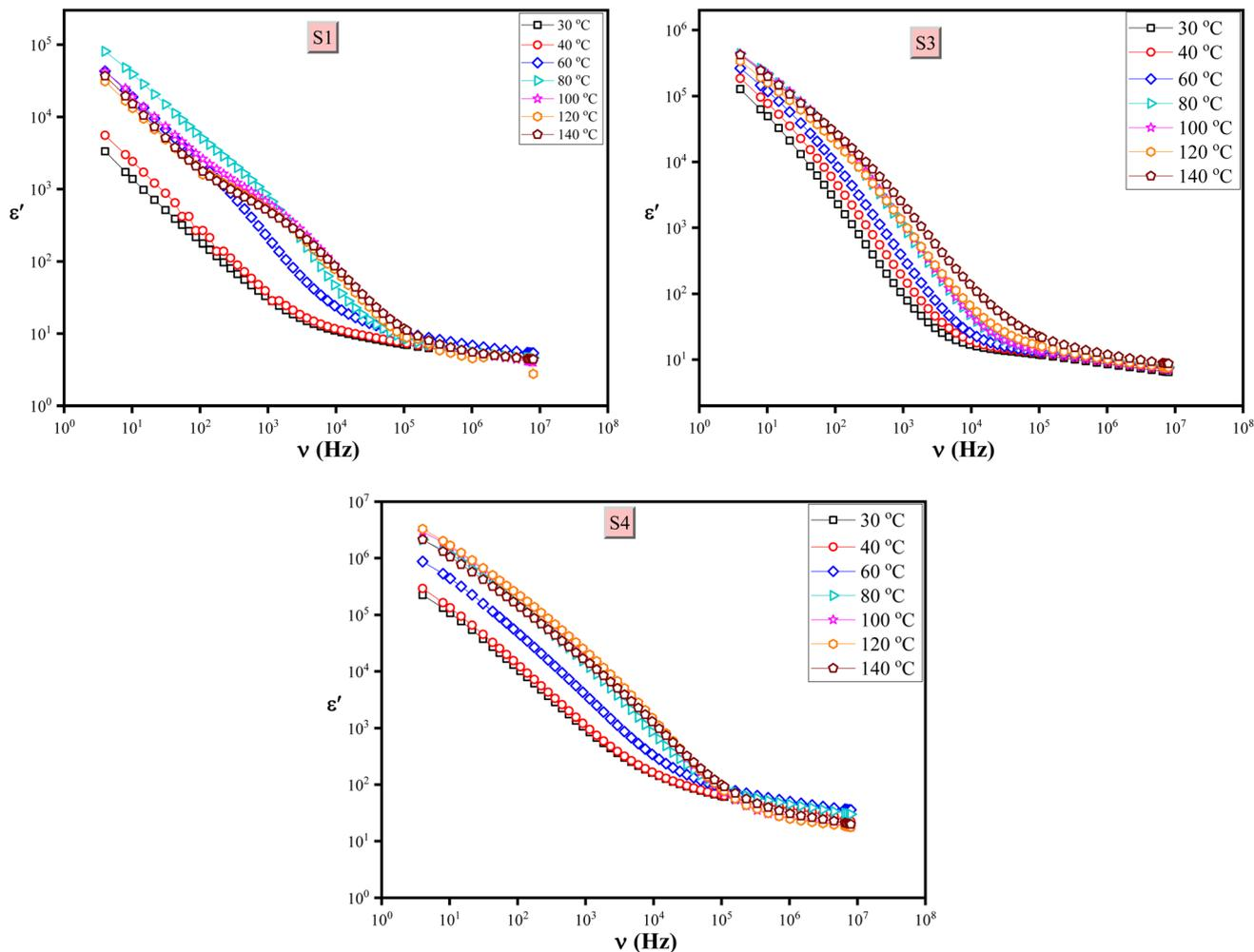
Fig. 5 Dielectric constant ( $\epsilon'$ ) of HEC and HEC@  $\text{ZnCe}_{0.3}\text{Ti}_{0.7}\text{O}_3$  nanocomposites (S1, S3, and S4) at different temperatures (30 °C to 140 °C).
