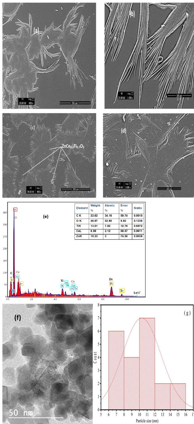
Fig. 3 SEM images (a–d) of HEC (S1) and HEC@ZnCe<sub>0.3</sub>Ti<sub>0.7</sub>O<sub>3</sub> nanocomposite (S3). (e) EDX pf sample S3, (f) TEM imag of S3, and (g) is the particle distribution of ZnCe<sub>0.3</sub>Ti<sub>0.7</sub>O<sub>3</sub> NPs.
