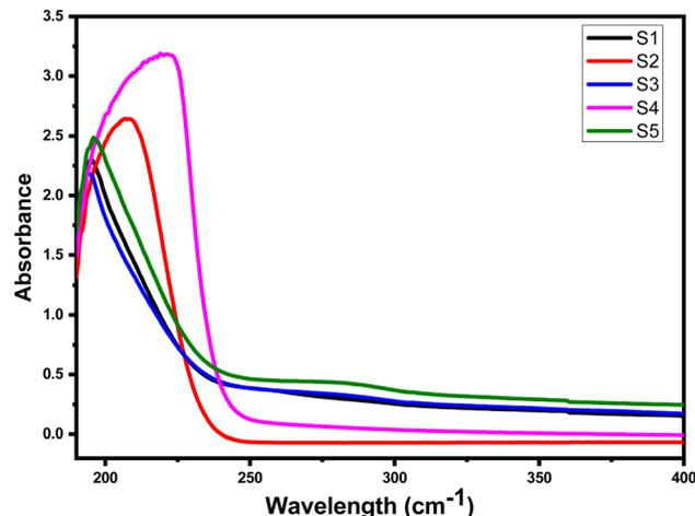
Fig. 4 UV-absorbance of HEC and HEC@ZnCe<sub>0.3</sub>Ti<sub>0.7</sub>O<sub>3</sub> nanocomposites.
