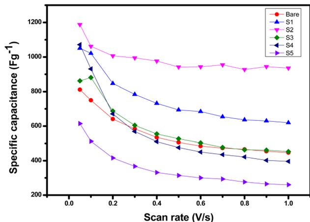
Fig. 12 Linearity curve between specific capacitance values vs. scan rate of unmodified bare and modified screen-printed electrodes with HEC and HEC@ZnCe<sub>0.3</sub>Ti<sub>0.7</sub>O<sub>3</sub> nanocomposites.
