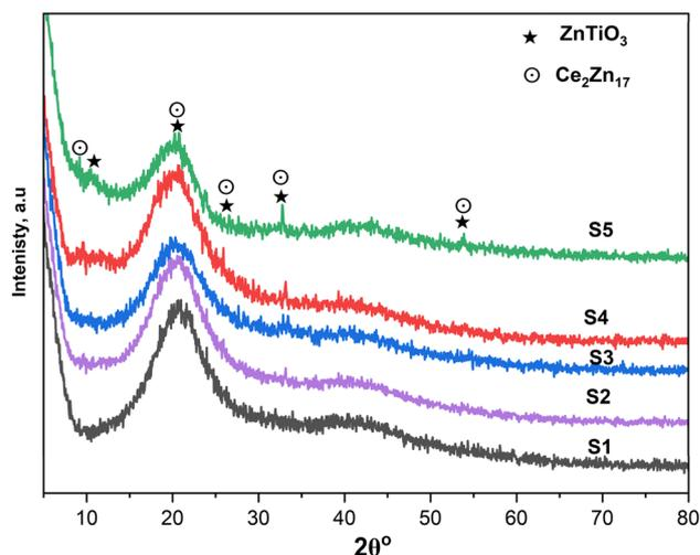
Fig. 2 XRD patterns of HEC (S1) and HEC@ZnCe<sub>0.3</sub>Ti<sub>0.7</sub>O<sub>3</sub> nanocomposites (S3, S4, and S5).
