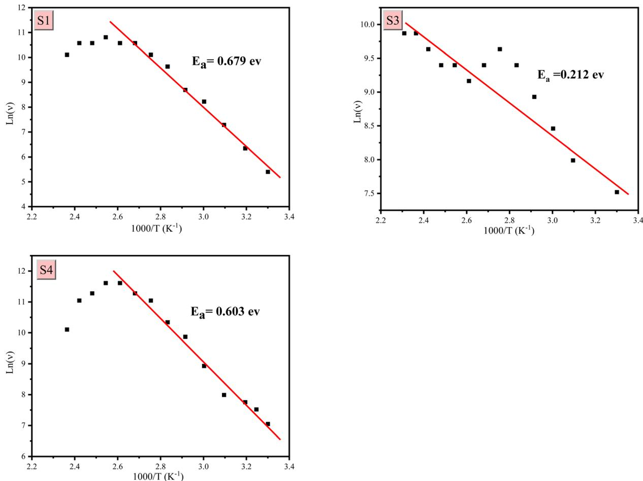
Fig. 7 Arrhenius plots of  $\ln(\nu)$  versus  $1000/T$  for HEC and HEC@ZnCe<sub>0.3</sub>Ti<sub>0.7</sub>O<sub>3</sub> nanocomposites (S1, S3, and S4).
