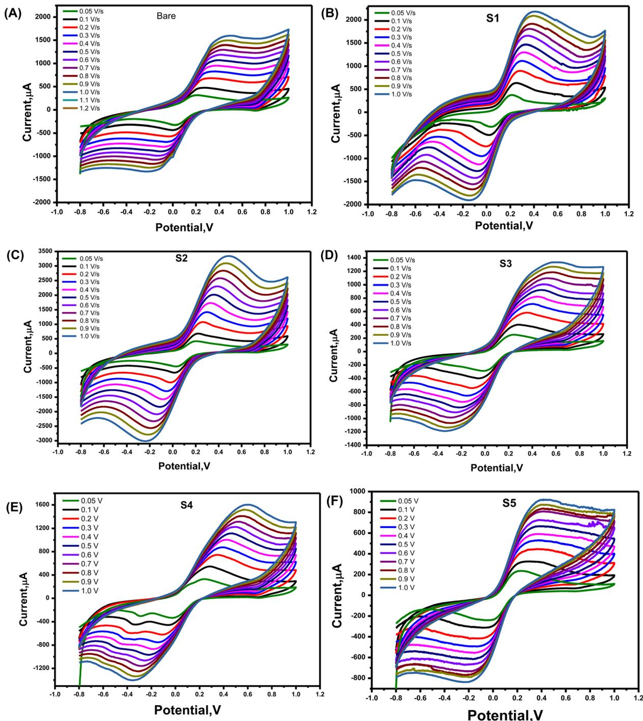
Fig. 10 Cyclic voltammograms of (A) Bare, (B) S1, (C) S2, (D) S3 (E) S4, and (F) S5 modified screen printed electrodes at different scan rates from 50–1000  $\text{mV s}^{-1}$  in a solution containing 5 mM ferro/ferricyanide and 0.1 M KCl.
