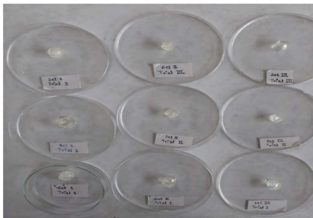
Fig. 1 Physical appearance of dried hydrogel discs.
