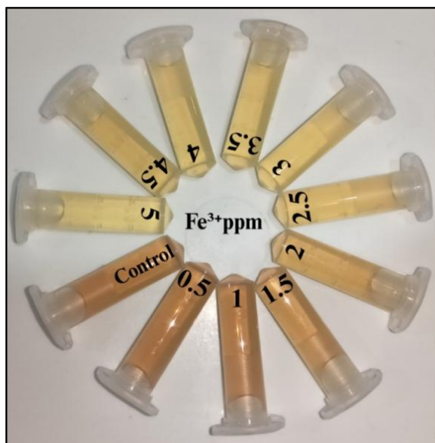
Fig. 19 \text{Fe}^{3+} -AgNPs interactions: visual color change of AgNPs solutions with increasing \text{Fe}^{3+} concentration (0.5–5 ppm).
