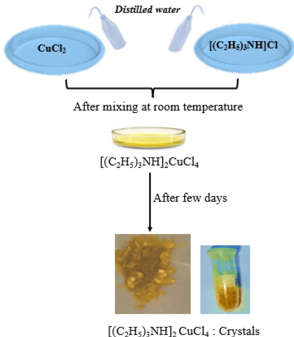
Fig. 1 Synthesis of  $[(\text{C}_2\text{H}_5)_3\text{NH}]_2\text{CuCl}_4$  single crystals.
