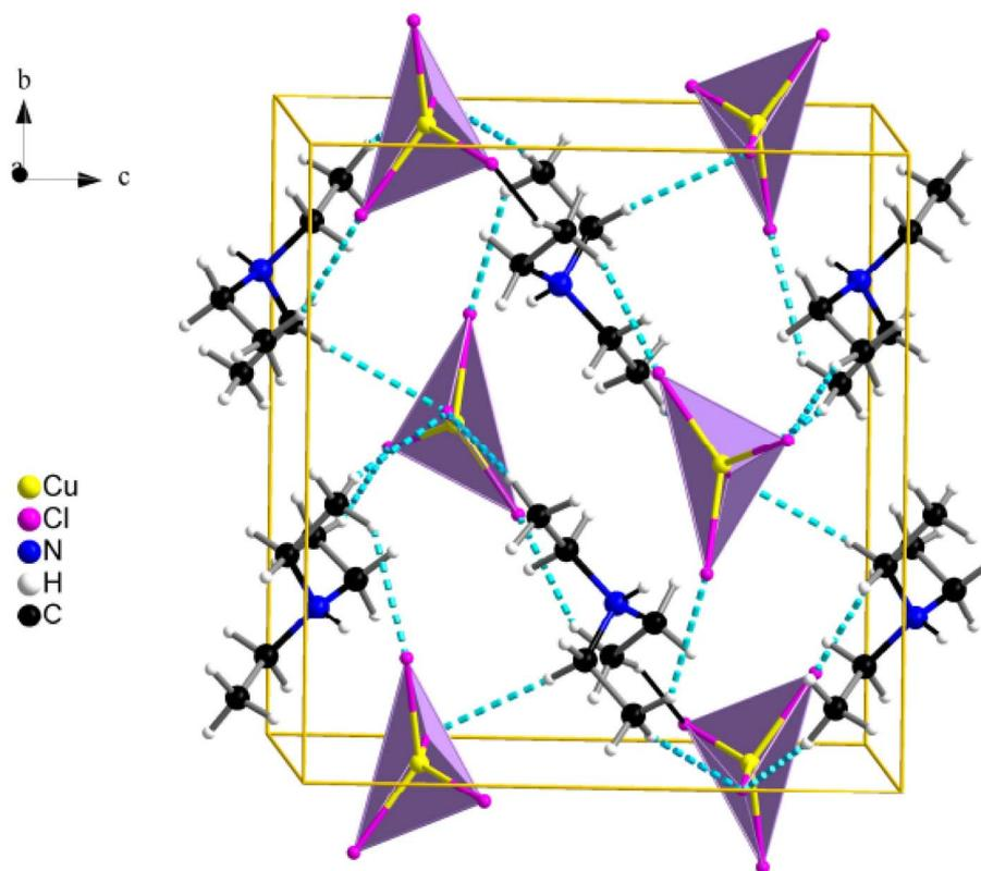
Fig. 3 Crystal packing arrangement of  $[(\text{C}_2\text{H}_5)_3\text{NH}]_2\text{CuCl}_4$  compound.
