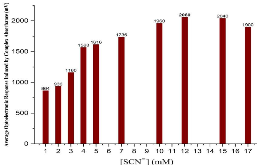
Fig. 5 The effect of the SCN<sup>-</sup> concentration on photocurrent response, confirming the optimal value at 12 mM.
