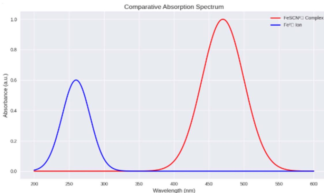
Fig. 3 UV-Vis absorption profiles of the  $\text{FeSCN}^{2+}$  complex ( $\lambda_{\text{max}} = 470 \text{ nm}$ ) and free  $\text{Fe}^{2+}$  ions ( $\lambda_{\text{max}} \approx 260 \text{ nm}$ ), illustrating the enhanced visible-region response of the coloured complex.
