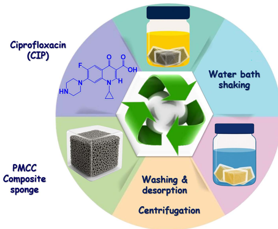
Fig. 2 Diagrammatic representation of the adsorption and removal of CIP by PMCC.
