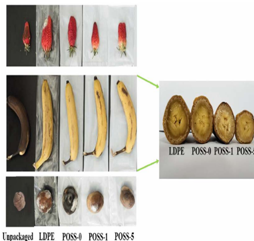
Fig. 11 (a) Schematic diagram of gas permeation in PBAT/PLA/POSS (epoxy) 8 films. (b) Photographs of strawberries, bananas, and mushrooms stored in air and in different types of plastic bags for 11 days. This figure has been reproduced from ref. 137 with permission from Food Chemistry , Copyright 2021.
