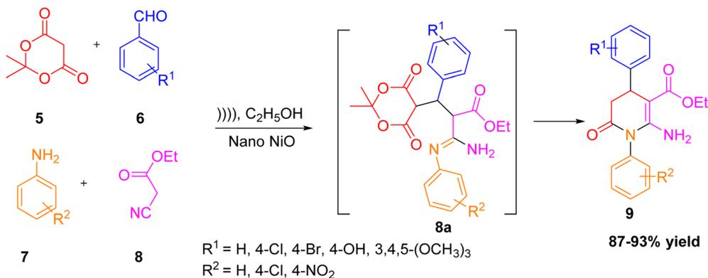
Scheme 2 Formation of tetrahydropyridine-3-carboxylates by using ultrasound irradiation.
