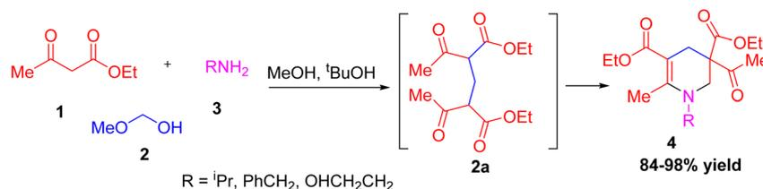
Scheme 1 Solvent selective multicomponent synthesis of monocyclic 1,2,3,4-tetrahydropyridine derivatives.
